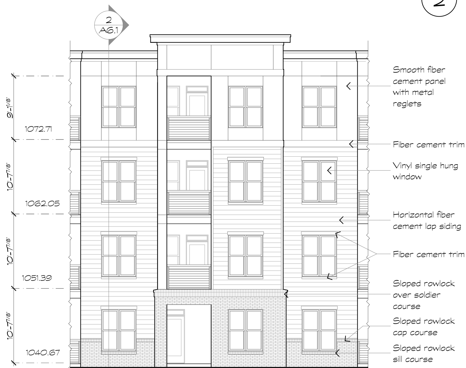
3 Courtyard Elevation Scale: 1/8" = 1'-0"
