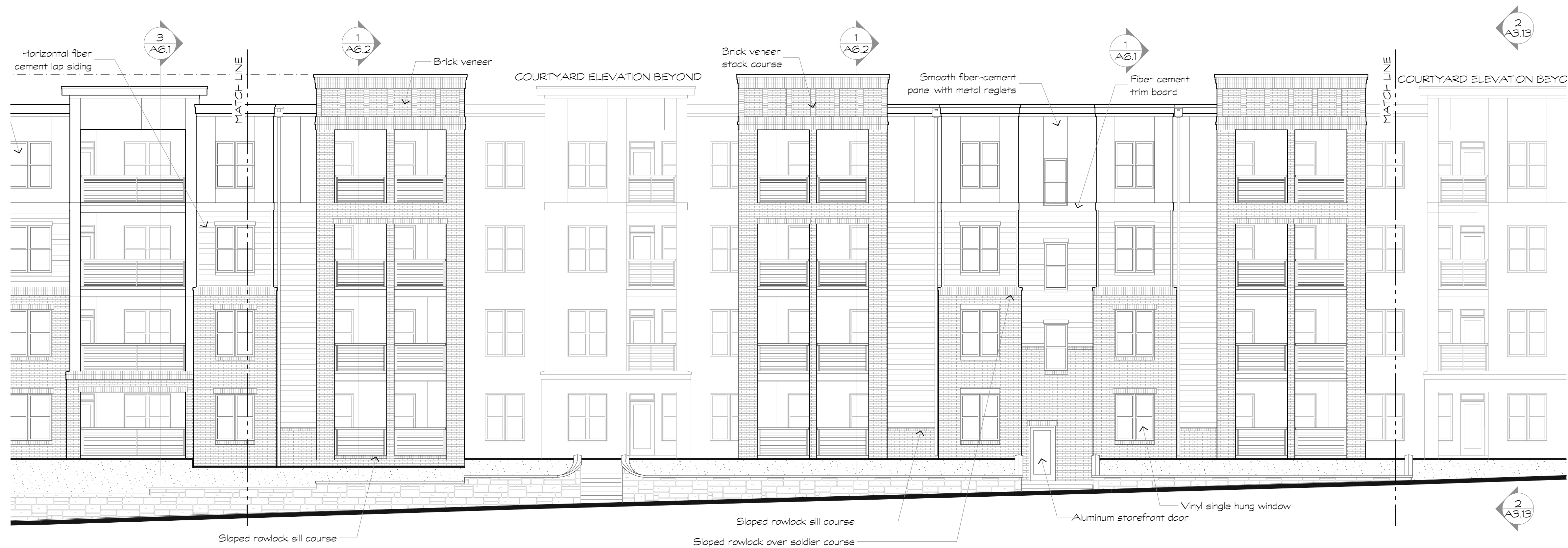
2 Building Elevation - SE Douglas Street Scale: 1/8" = 1'-0"
