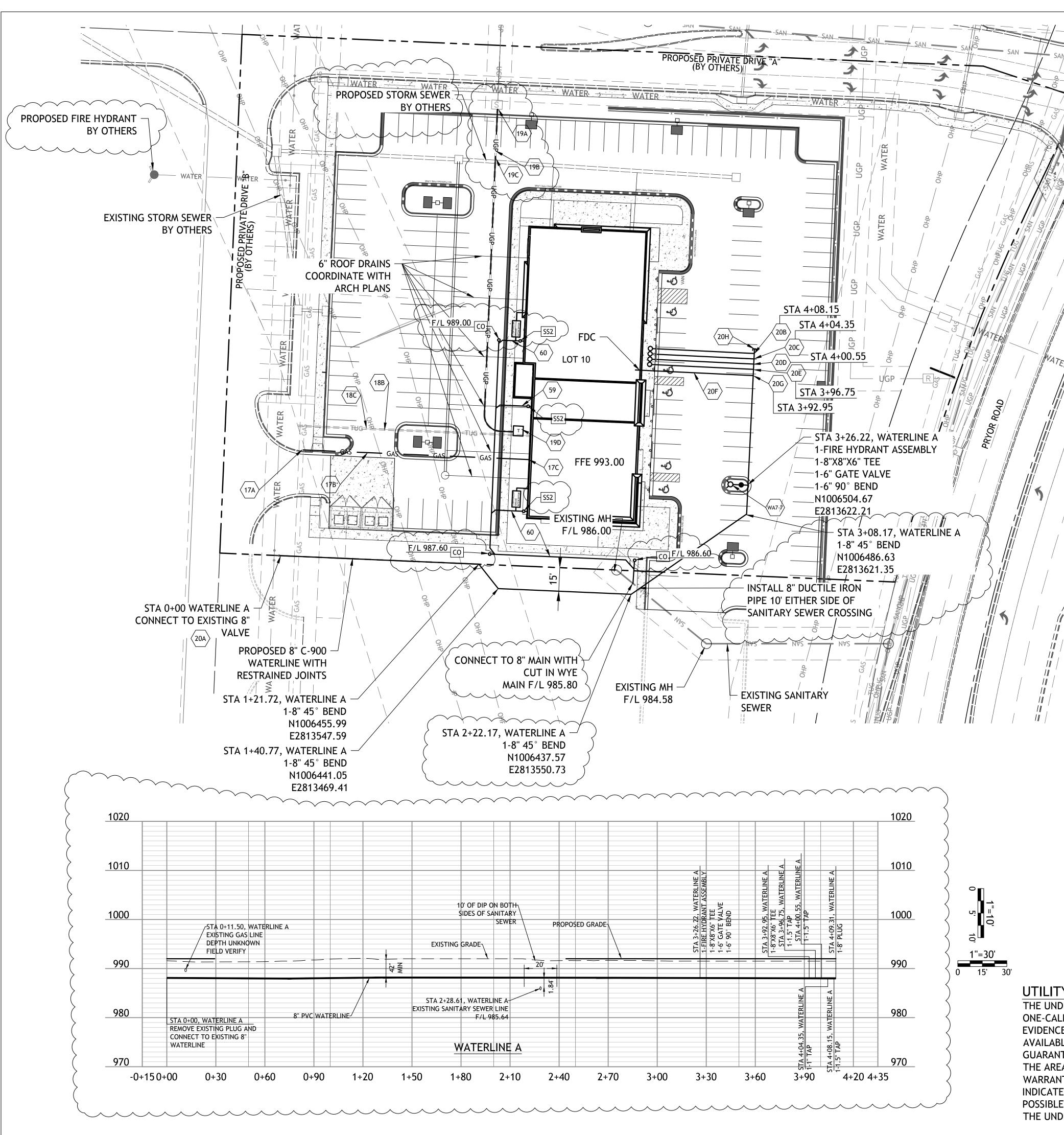
**UTILITY NOTES:** . ALL UTILITY AND STORM SEWER TRENCHES CONSTRUCTED UNDER AREAS THAT RECEIVE PAVING SHALL BE BACKFILLED TO 18 INCHES ABOVE THE TOP OF THE PIPE WITH SELECT GRANULAR MATERIAL PLACED ON EIGHT-INCH LIFTS, AND COMPACTED TO 95% MODIFIED PROCTOR DENSITY.
