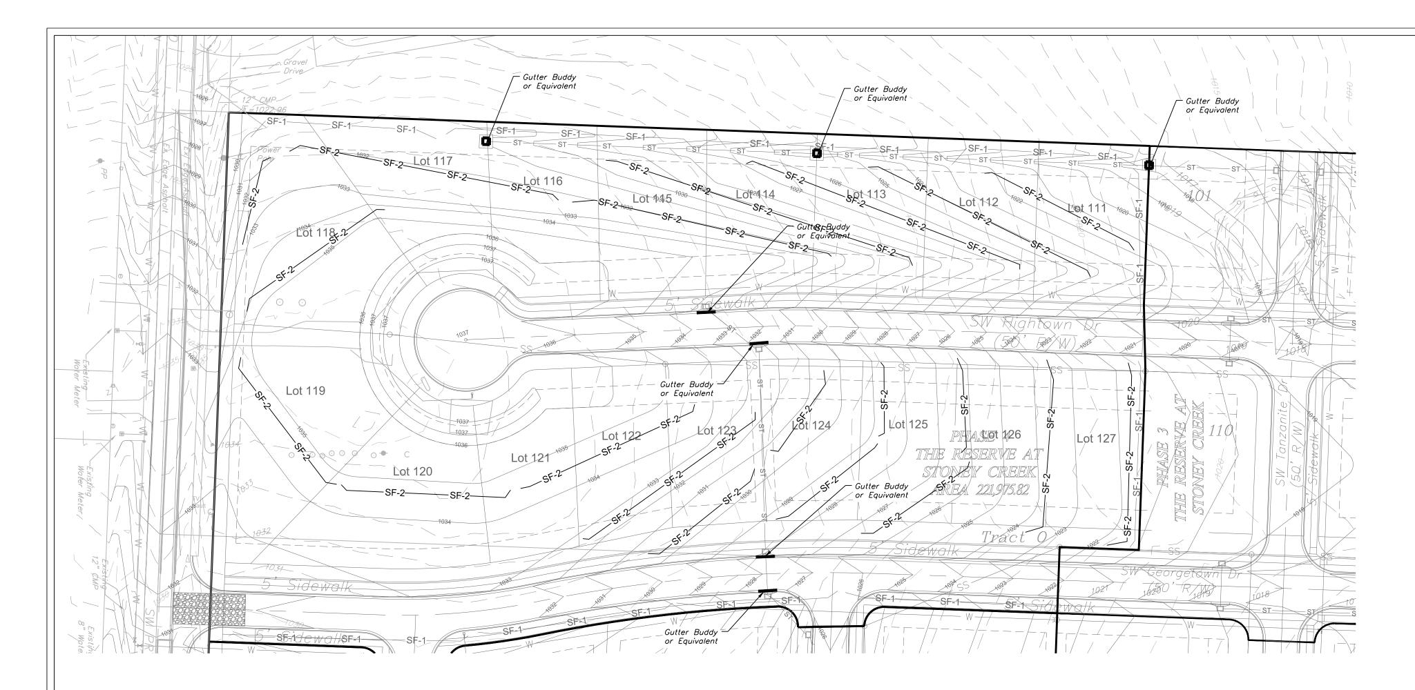
MAINTENANCE: TO MAINTAIN THE EROSION AND SEDIMENT CONTROLS, THE FOLLOWING PROCEDURES WILL BE PERFORMED: SEDIMENT CAPTURE DEVICES: SEDIMENT WILL BE REMOVED FROM THE UPSTREAM OR UPSLOPE SIDE OF THE FILTER FABRIC FENCES, WHEN THE DEPTH OF ACCUMULATED SEDIMENT REACHES ABOUT ONE-THIRD THE HEIGHT OF THE STRUCTURE.
