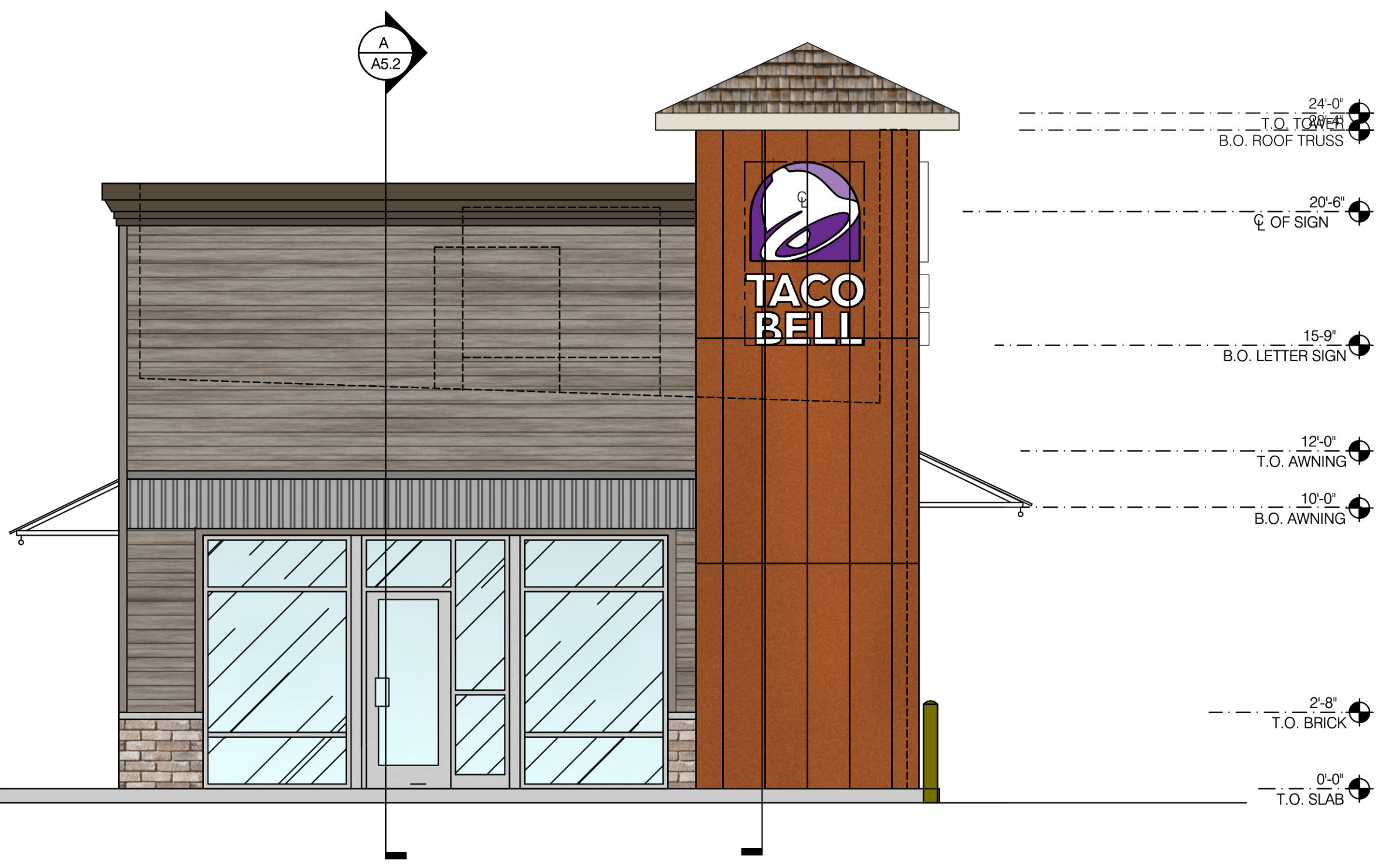
WEST ELEVATION 1/4" = 1'-0" C
