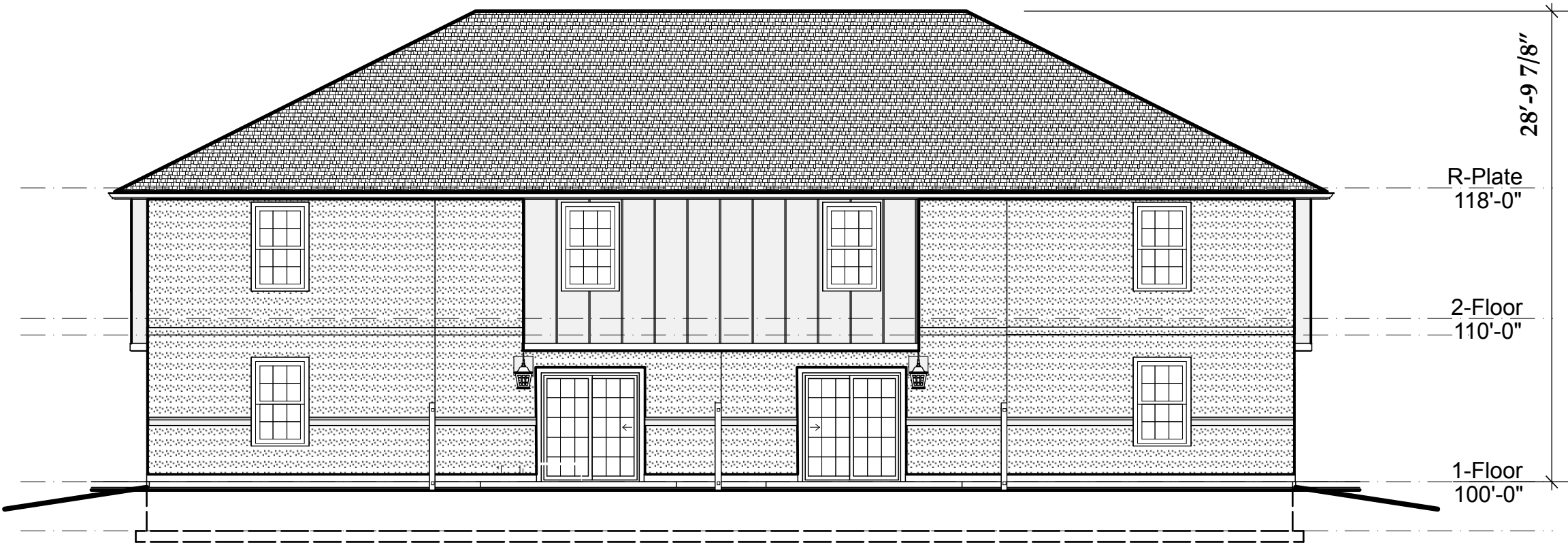
TYPICAL REAR ELEVATION Scale 1/8" = 1'-0"
