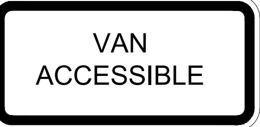
VAN ACCESSIBLE 6"x12" ACCESSIBLE SIGN DETAIL N.T.S.
