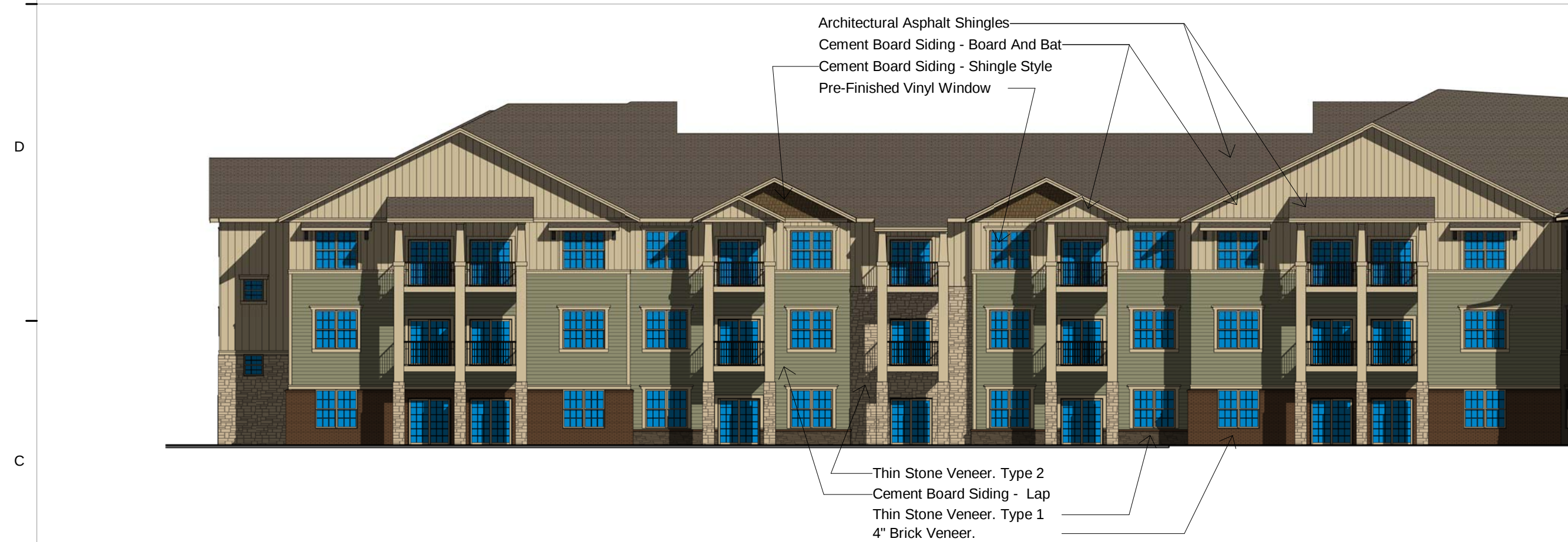
C10 PARTIAL WEST ELEVATION - IL NORTH 1/16" = 1'-0"
