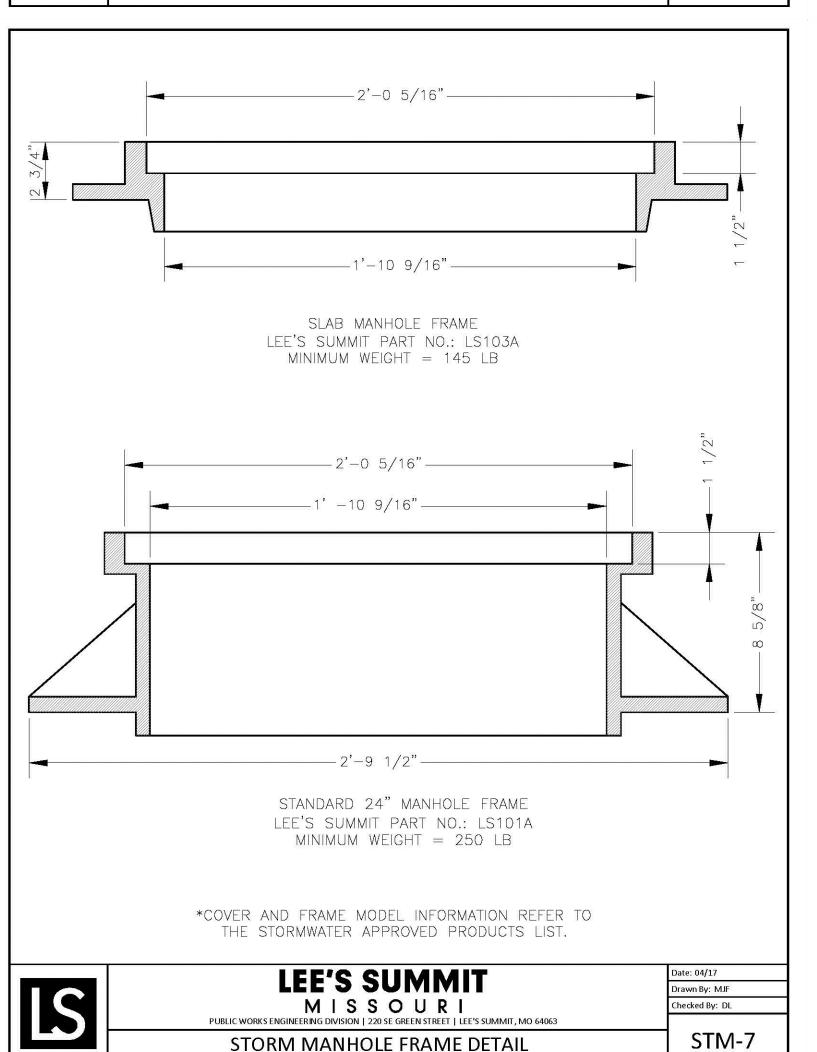
STORM MANHOLE FRAME DETAIL
