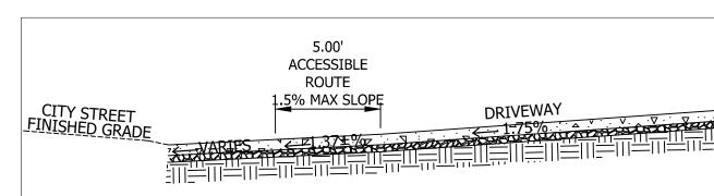
SECTION B- SECTION OF ACCESSIBLE PATH ON DRIVEWAY
