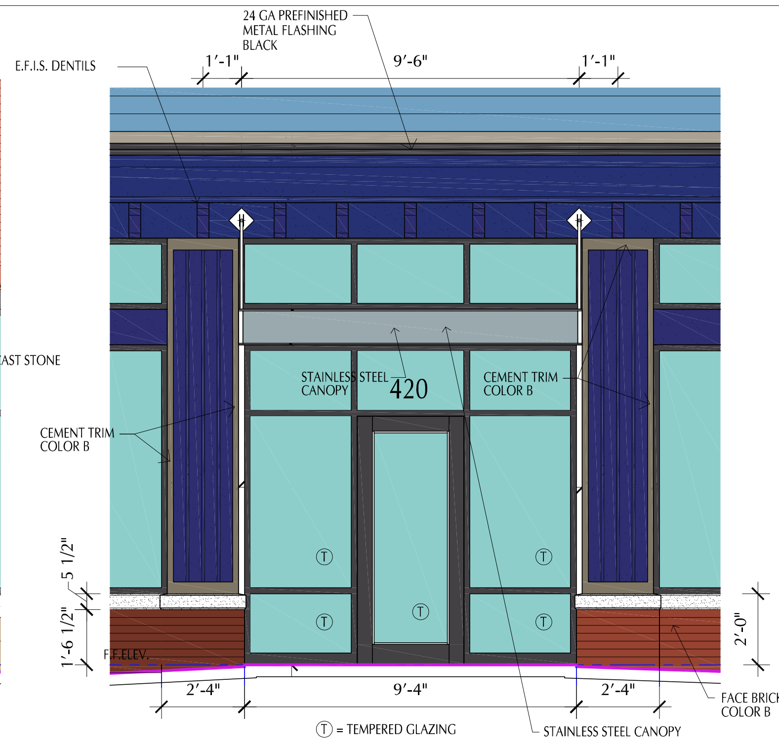
ENLARGED EAST ELEVATION 3 Scale 3/8" = 1'-0"
