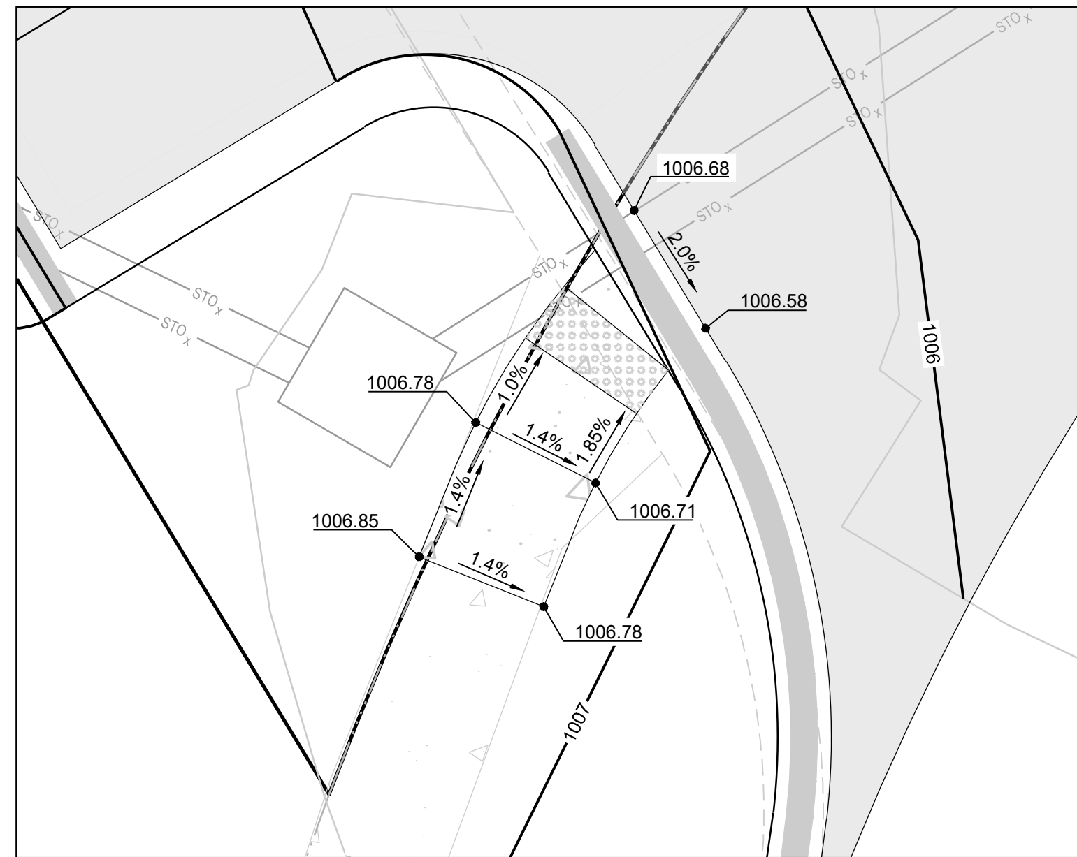
1. MAXIMUM SLOPE IN HANDICAPPED PARKING STALLS SHALL BE 2% (1:50 IN ALL DIRECTIONS). 2. MAXIMUM SIDEWALK CROSS SLOPE SHALL BE 2.0% (1:50).
