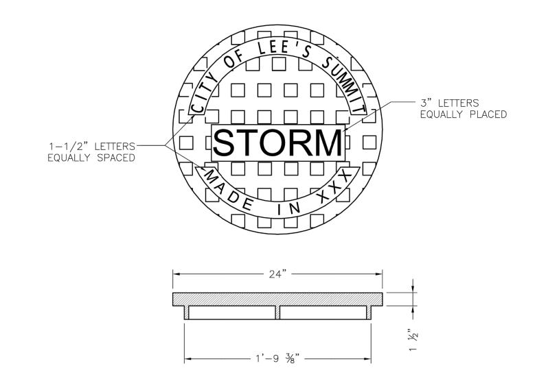
STANDARD 24" MANHOLE COVER MINIMUM WEIGHT = 160 LB NOTE: PICK HOLES NOT SHOWN
