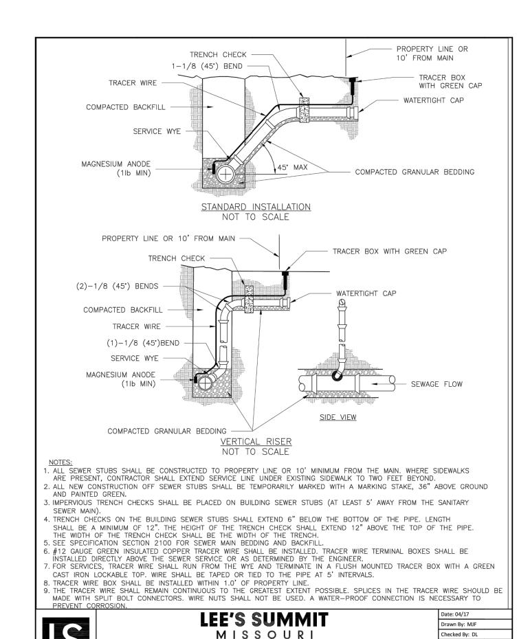
**BUILDING SEWER STUB AND RISER**
