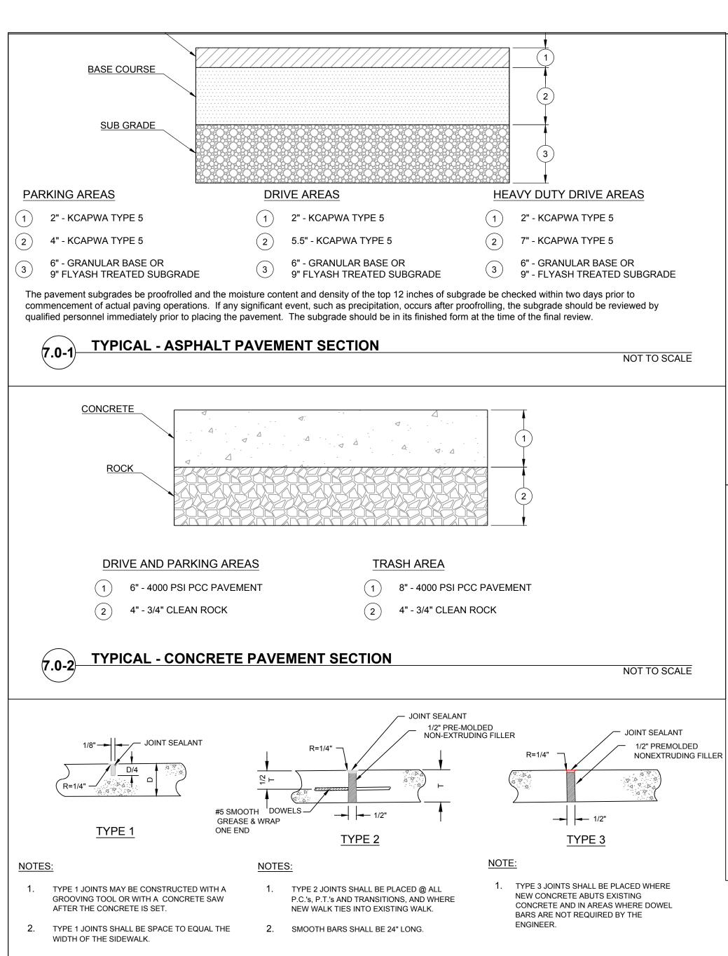
**TYPICAL - CONCRETE PAVEMENT JOINT DETAILS**
