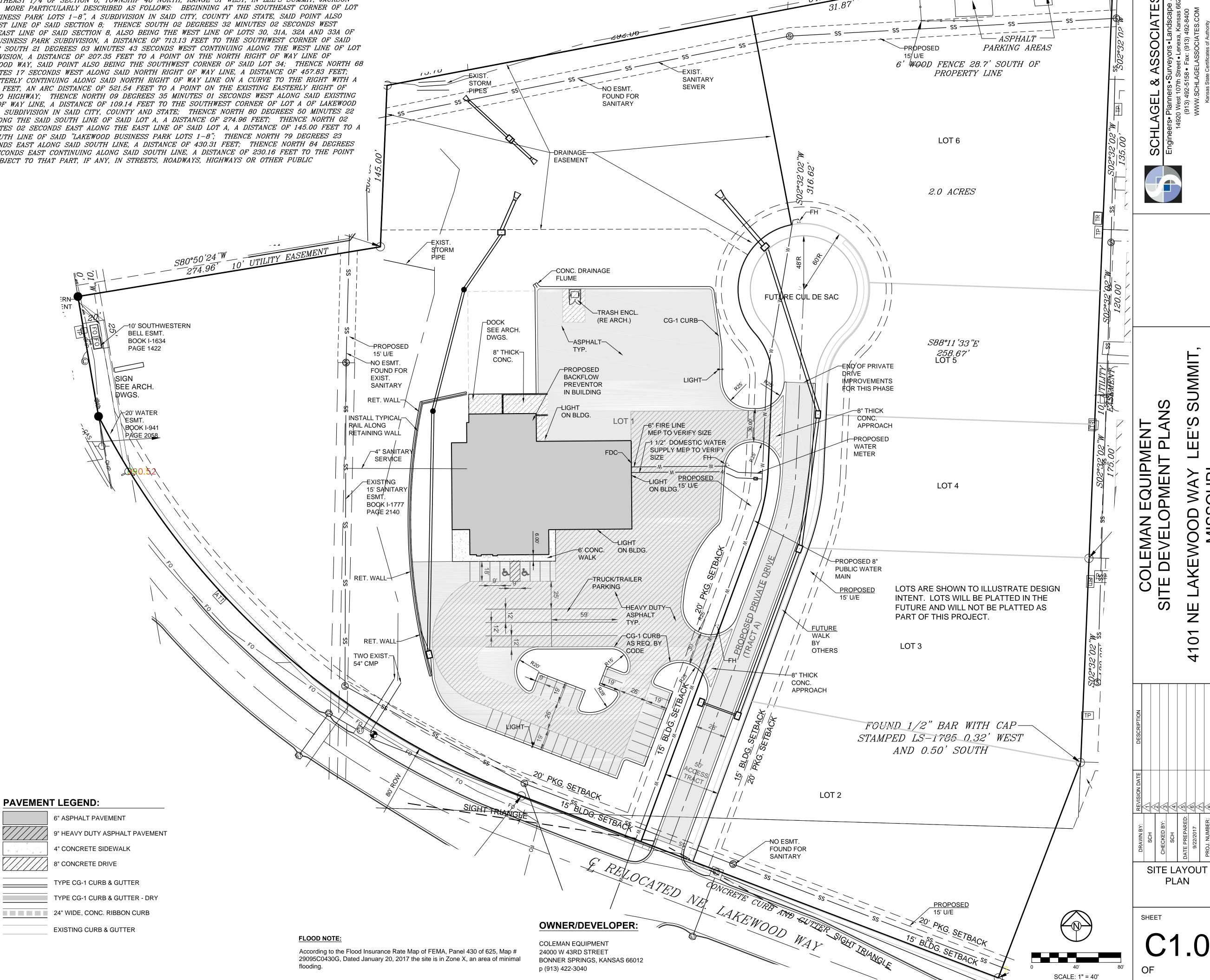
ADDEMDUM #1 PLAN CHANGES STORM PIPE ALONG PRIVATE STREET MODIFIED STORM PIPE SIZES ADDED 3. THE NORTH ENTRANCE WIDTH WAS REDUCED. 4. ALL GATES WERE REVISED 5. A 42" GUARD RAIL WAS ADDED ALONG THE TOP OF THE WALL ALONG THE CREEK
