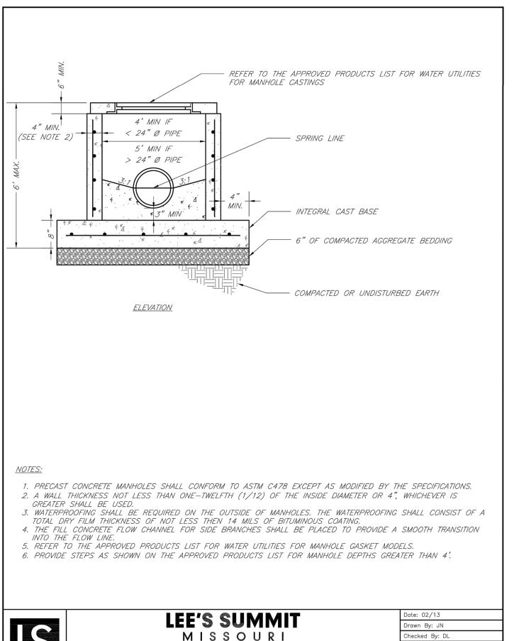
SHALLOW PRECAST MANHOLE - SANITARY SEWER
