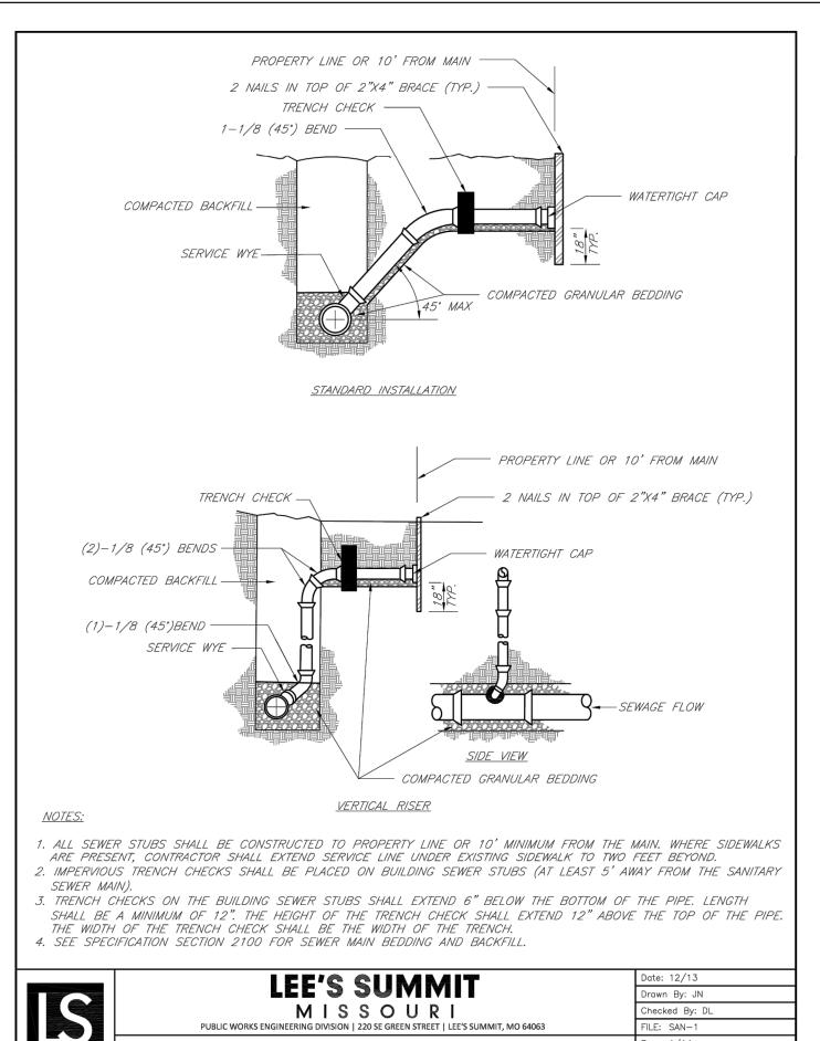
BUILDING SEWER STUB AND RISER
