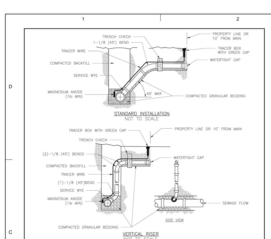
1. ALL SEWER STUBS SHALL BE CONSTRUCTED TO PROPERTY LINE OR 10' MINIMUM FROM THE MAIN. WHERE SIDEWALKS ARE PRESENT, CONTRACTOR SHALL EXTEND SERVICE LINE UNDER EXISTING SIDEWALK TO TWO FEET BEYOND.
