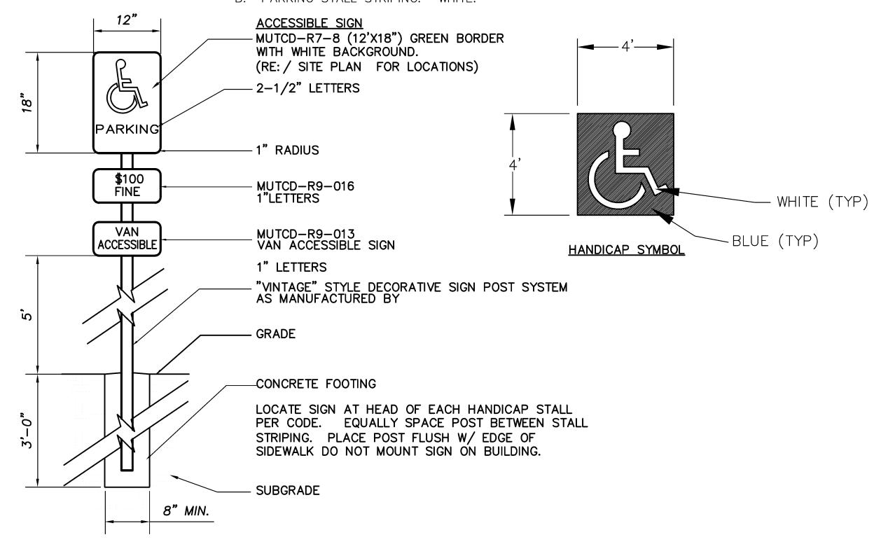
HANDICAPPED SIGNAGE & PAVEMENT MARKING DETAIL
