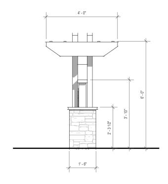
ELEVATION SHOWN FLAT. DESIGN CURVED IN PLAN.
