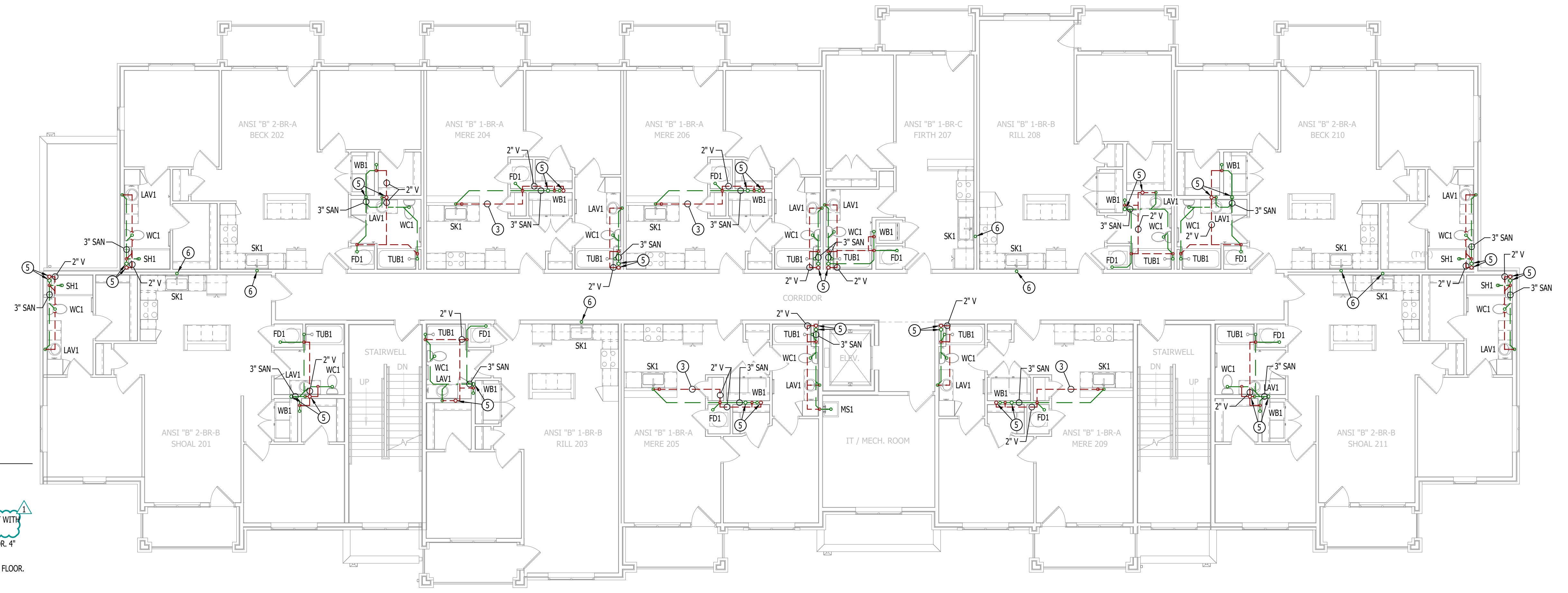
SANITARY SEWER PLAN - SECOND FLOOR SCALE: 1/8" = 1'-0"
