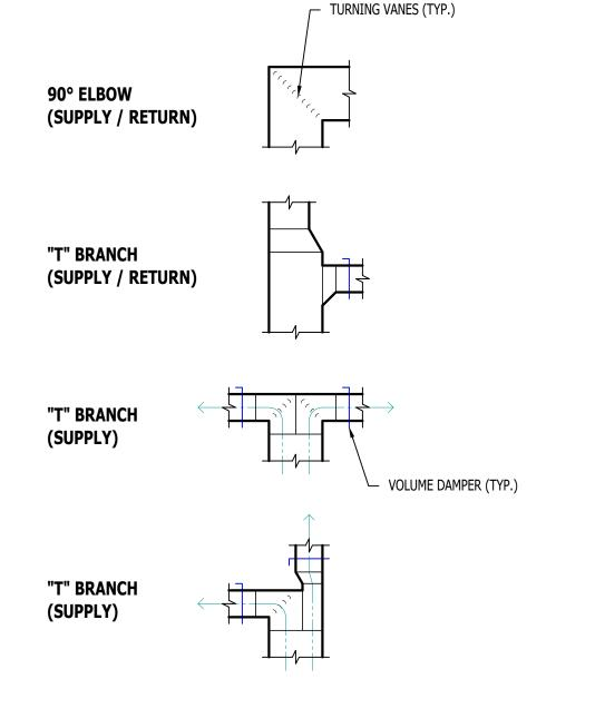
TYPICAL DUCTWORK FITTINGS DETAIL
