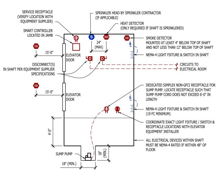
**MACHINE - ROOM - LESS ELEVATOR DETAIL**
