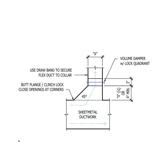
TYPICAL DUCTWORK DETAIL
