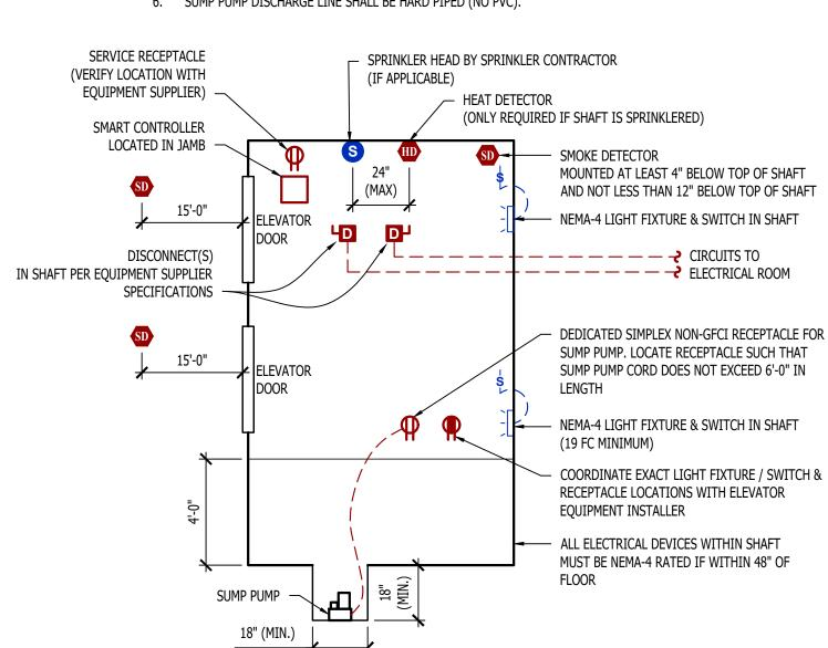
**MACHINE - ROOM - LESS ELEVATOR DETAIL**
