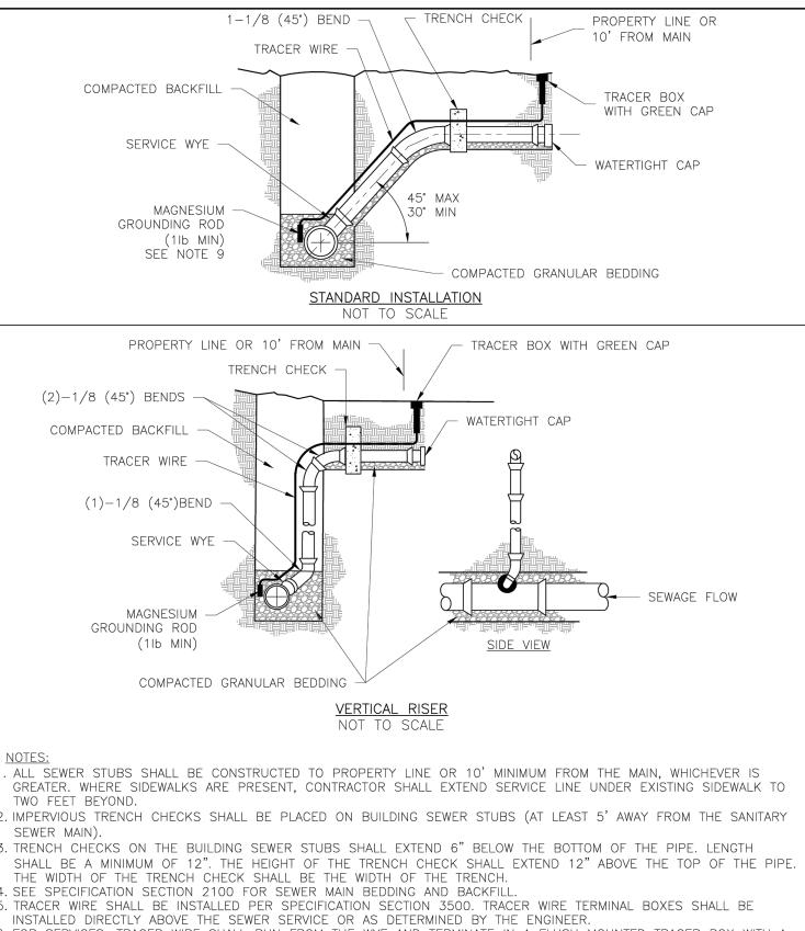
6. FOR SERVICES, TRACER WIRE SHALL RUN FROM THE WYE AND TERMINATE IN A FLUSH MOUNTED TRACER BOX WITH A GREEN CAST IRON LOCKABLE TOP. WIRE SHALL BE TAPED OR TIED TO THE PIPE AT 5' INTERVALS. . TRACER WIRE BOX SHALL BE INSTALLED WITHIN 1.0' OF PROPERTY LINE. 8. THE TRACER WIRE SHALL REMAIN CONTINUOUS TO THE GREATEST EXTENT POSSIBLE. SPLICES IN THE TRACER WIRE
