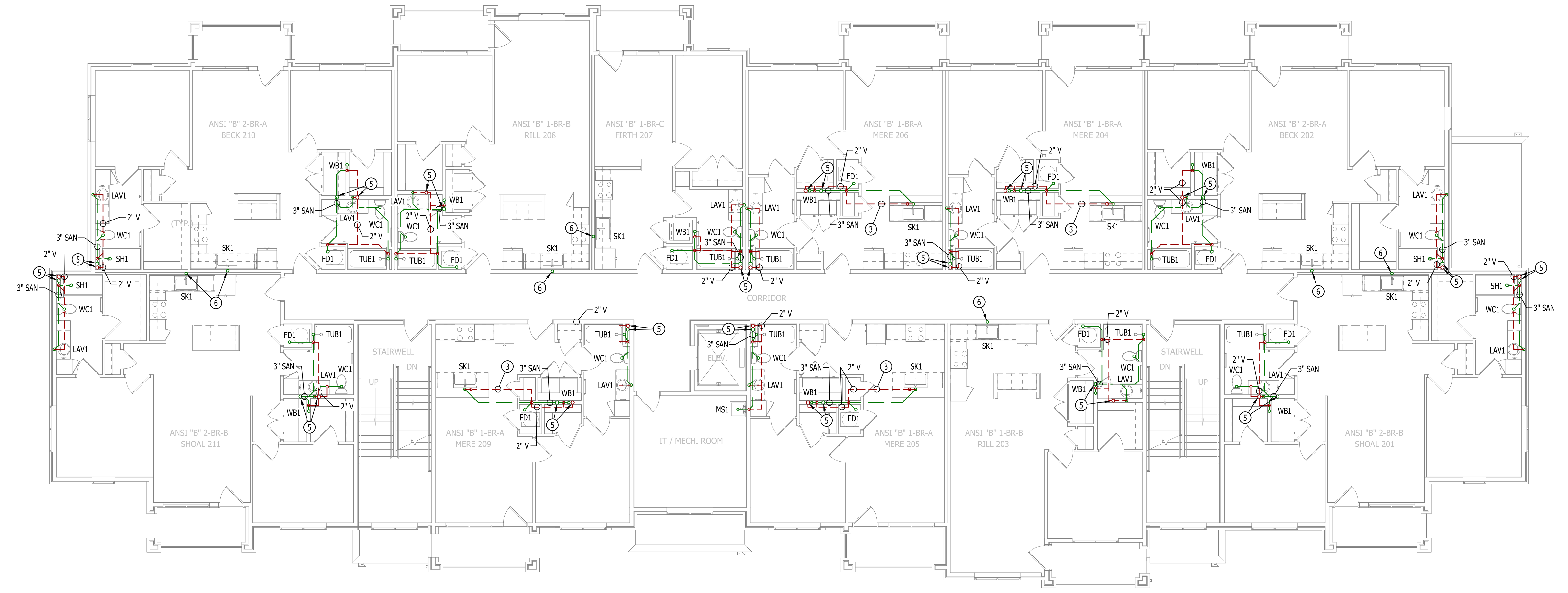
SANITARY SEWER PLAN - SECOND FLOOR SCALE: 1/8" = 1'-0"
