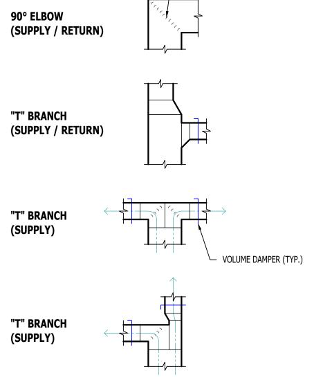
TYPICAL DUCTWORK FITTINGS DETAIL
