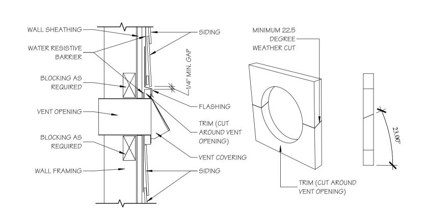
DRYER VENT IN SIDING DETAIL
