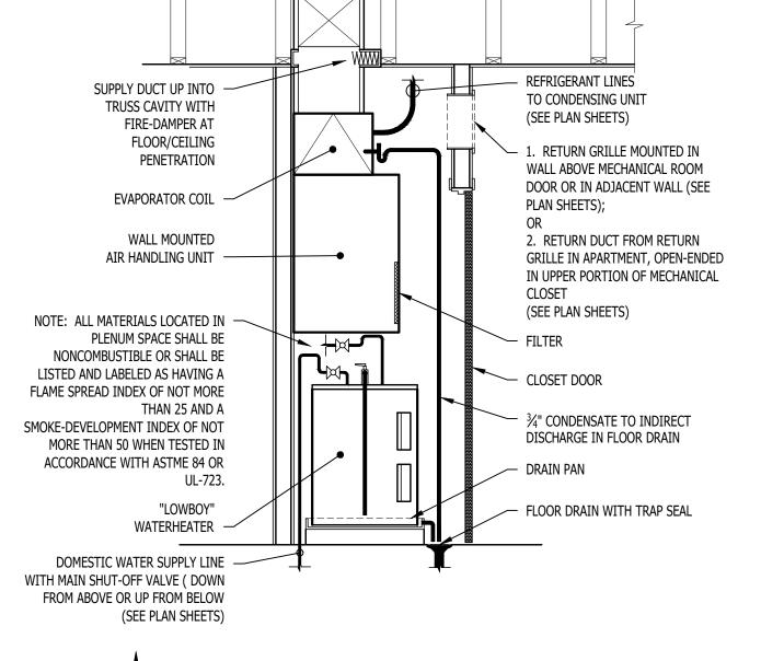
STACKED WATER HEATER / AHU DETAIL
