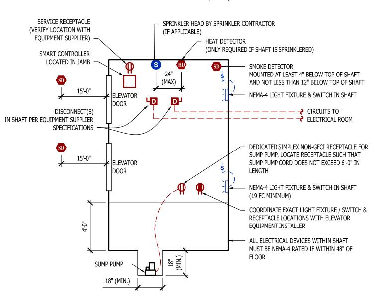
MACHINE - ROOM - LESS ELEVATOR DETAIL
