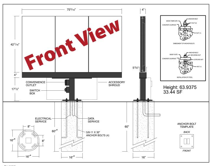
\*NOTE: These are approximate foundation measurements. The soil bearing capacity at the erection site must be considered when designing the foundation. The sign manufacturer is not able to predetermine the specific needs of each location. Consult a local engineer for design specifications.
