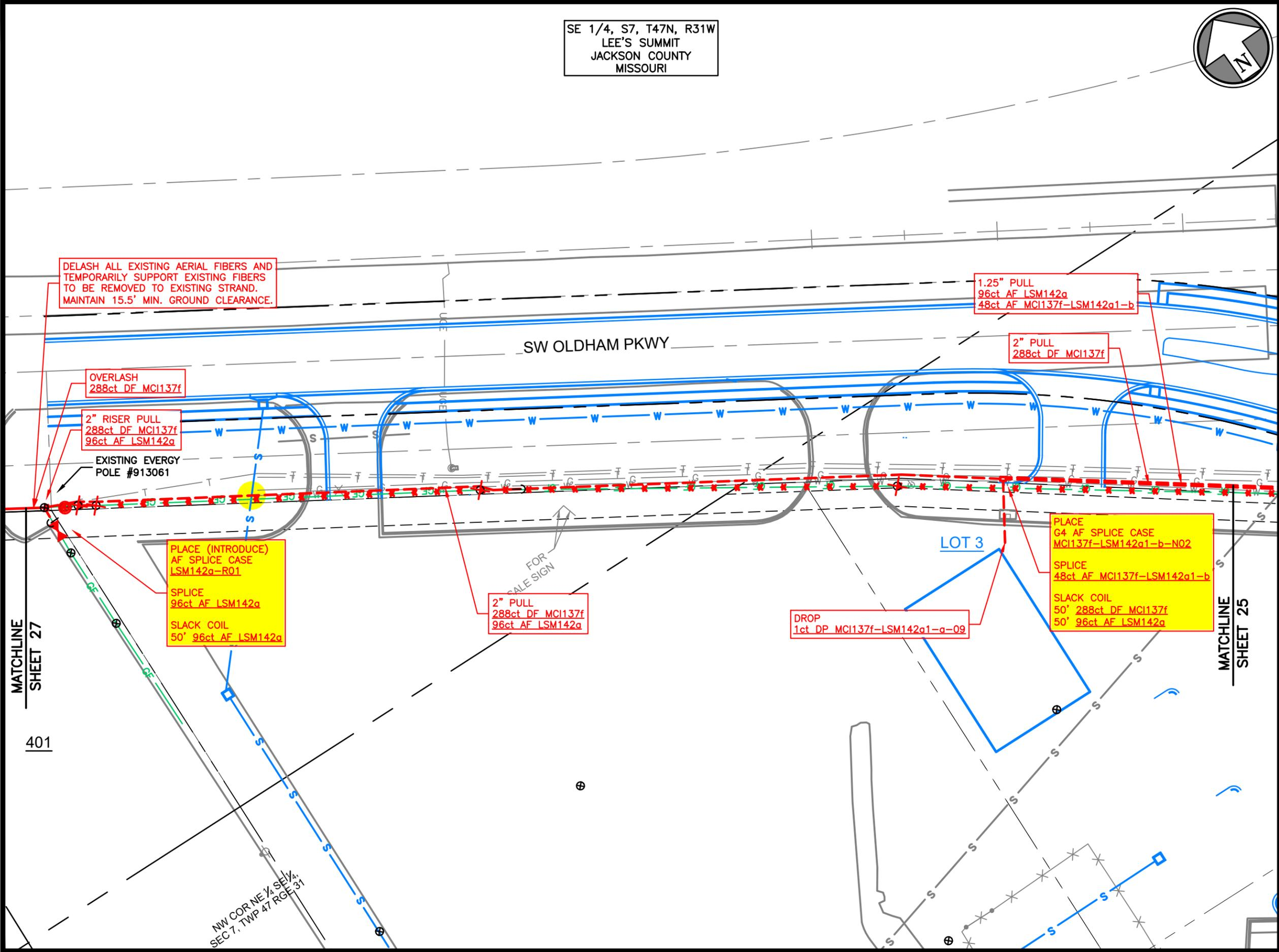
DELASH ALL EXISTING AERIAL FIBERS AND TEMPORARILY SUPPORT EXISTING FIBERS TO BE REMOVED TO EXISTING STRAND. MAINTAIN 15.5' MIN. GROUND CLEARANCE.
