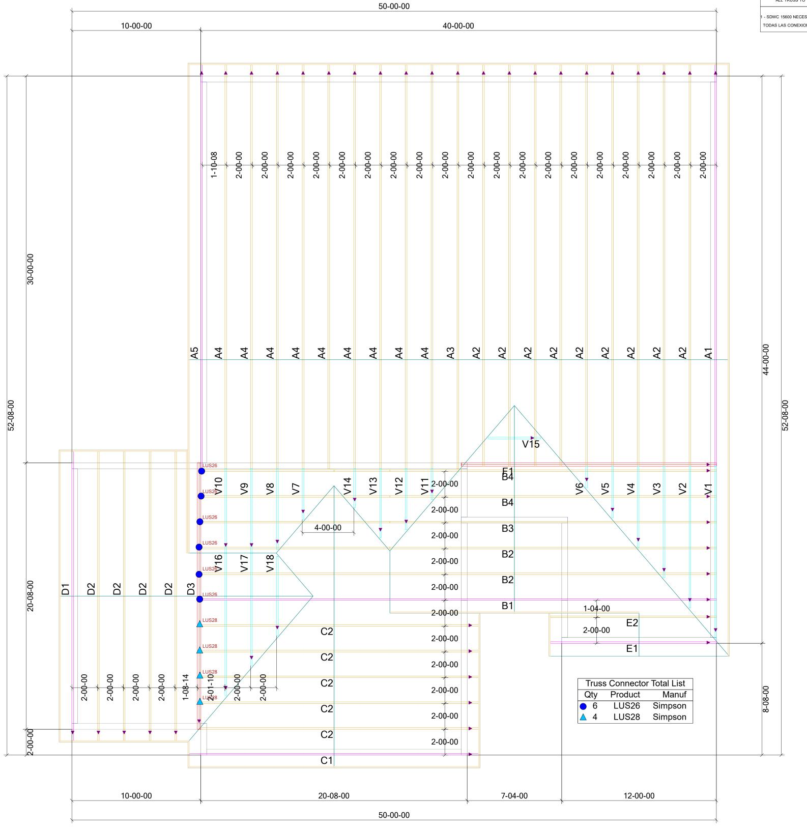
1 - SDWC 15600 REQUIRED AT ALL BEARING LOCATIONS (u.n.o.) ALL TRUSS TO TRUSS CONNECTIONS = 'NAILED'' (u.n.o.)
