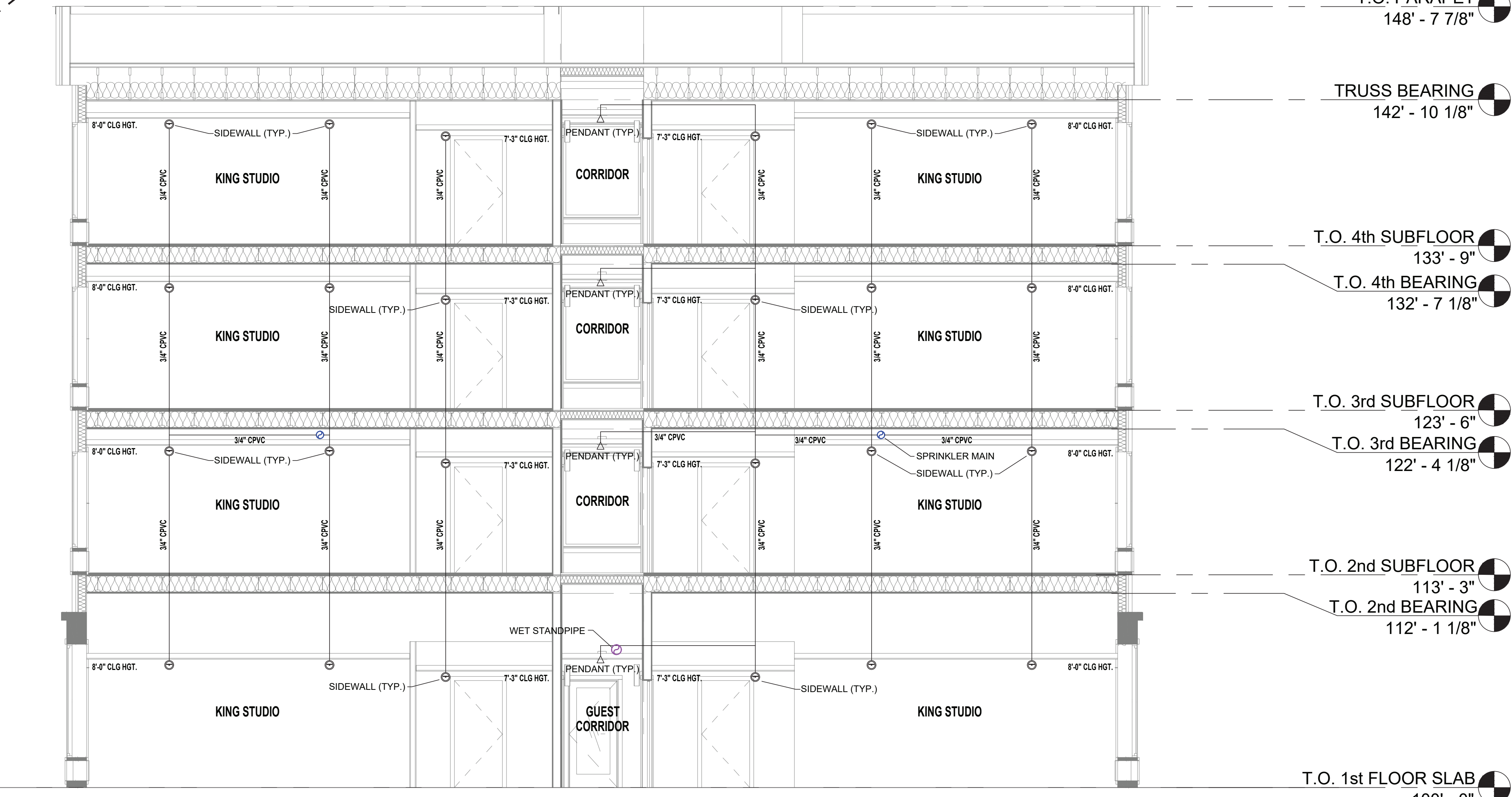
BUILDING CROSS SECTION
