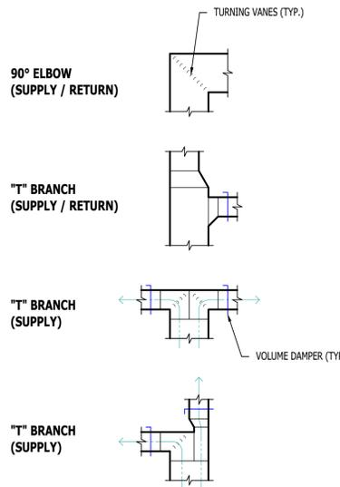
**TYPICAL DUCTWORK FITTINGS DETAIL**
