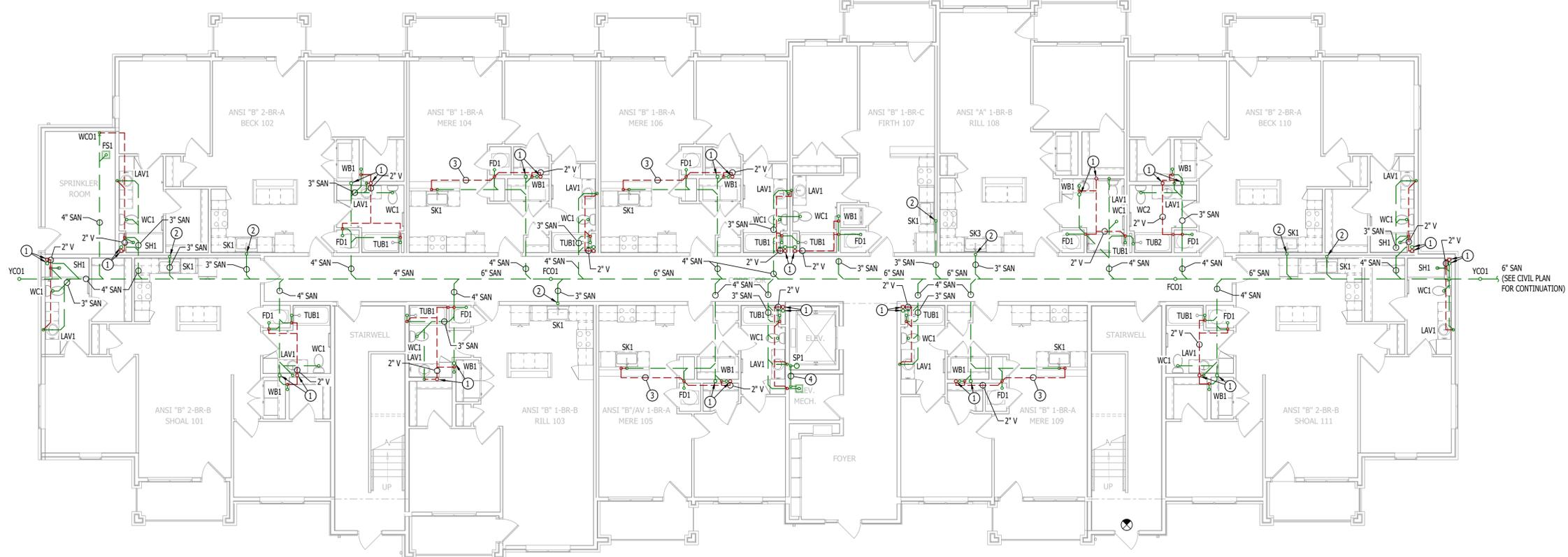
**SANITARY SEWER PLAN - FIRST FLOOR**
