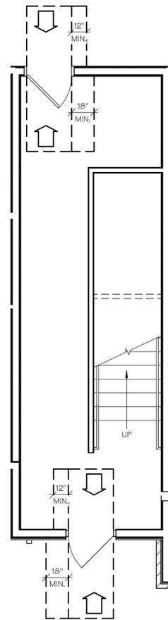
1ST FLOOR LEFT SIDE STAIRWELL ACC. PLAN
