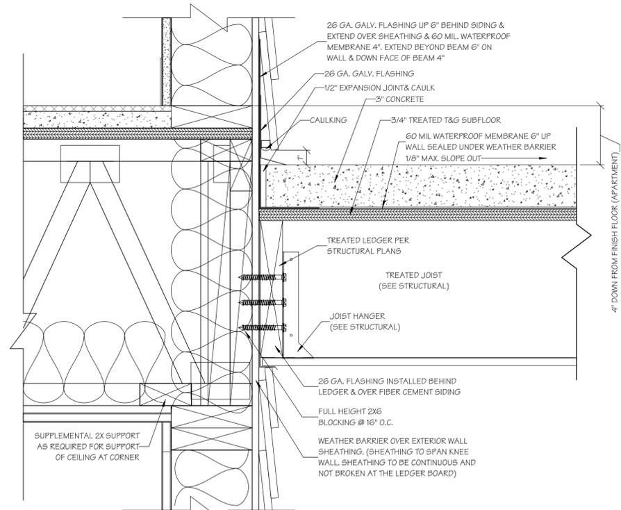
10 DECK FLASHING DETAIL
