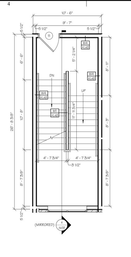
**2ND FLOOR RIGHT SIDE STAIRWELL DIM. PLAN**
