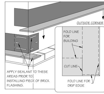
3 OUTSIDE CORNER FLASHING DETAIL @ BRICK
