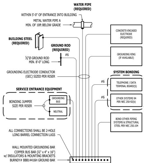
TYPICAL GROUNDING & BONDING DETAIL
