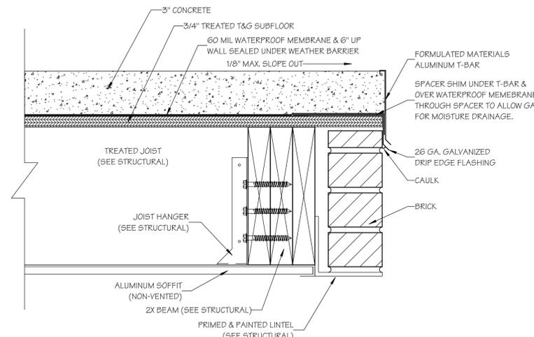
11 DECK EDGE FLASHING DETAIL
