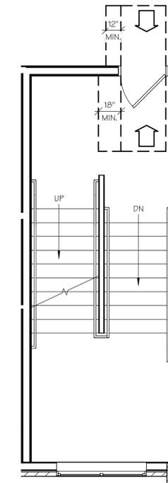
3RD FLOOR LEFT SIDE STAIRWELL ACC. PLAN
