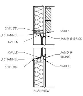
NOTE: WINDOWS W/ SIDING ABOVE REQUIRE FLASHING & CAULKING @ SIDING / FLANGE JUNCTION
