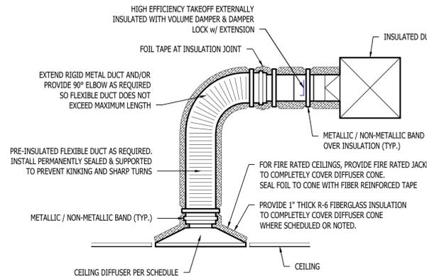
**TYPICAL LAY-IN DIFFUSER DETAIL**
