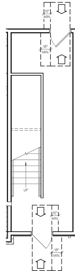
1ST FLOOR RIGHT SIDE STAIRWELL ACC. PLAN
