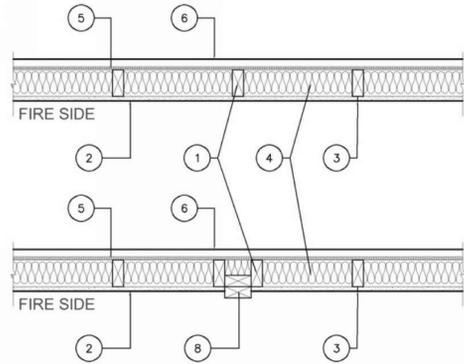
1. Wood Studs — Nom 2 by 4 in. spaced 16 in. OC with two 2 by 4 in. top and one 2 by 4 in. bottom plates. Studs laterally-braced by wood structural panel sheathing (Item 5). When Mineral and Fiber Boards\* (Item 5A) are considered as bracing for the studs, the load is restricted to 76% of allowable axial load. Walls effectively fire stopped at top and bottom of wall.
