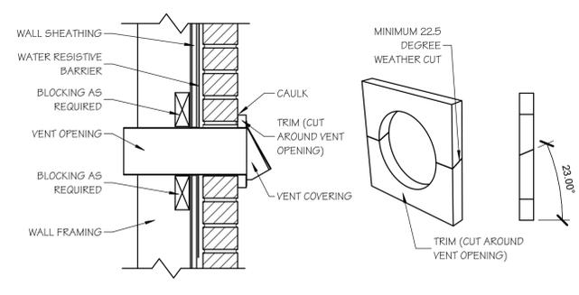
7 DRYER VENT IN BRICK DETAIL
