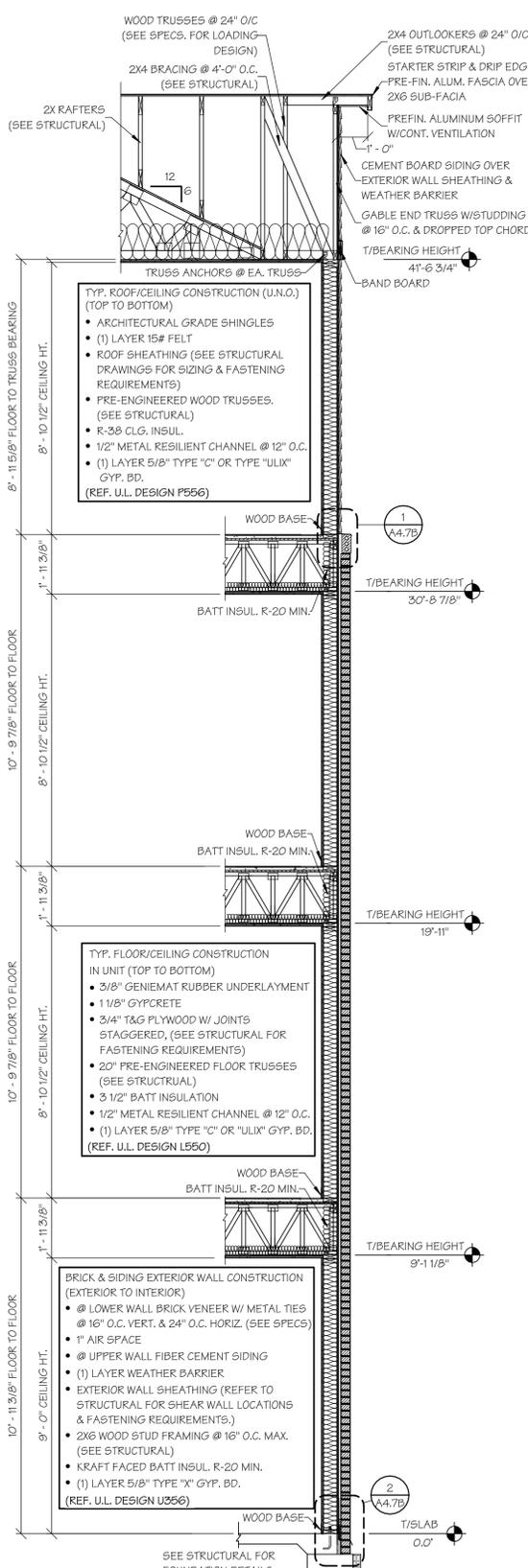
WALL SECTION WITH BRICK AND SIDING @ GABLE
