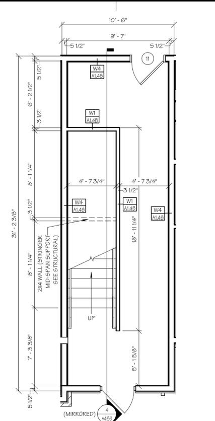
**1ST FLOOR RIGHT SIDE STAIRWELL DIM. PLAN**
