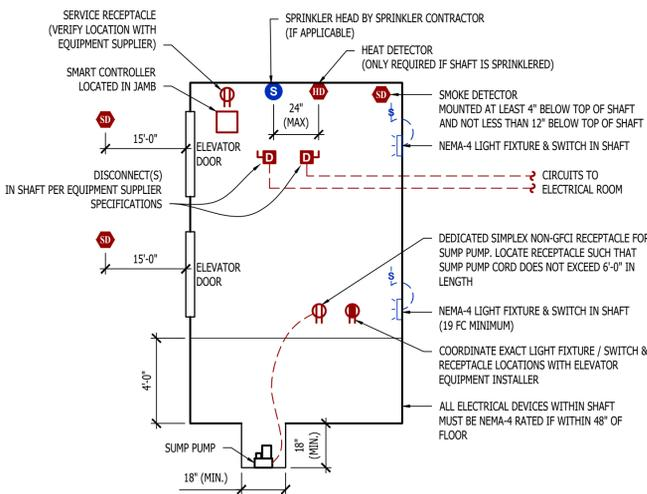
MACHINE - ROOM - LESS ELEVATOR DETAIL
