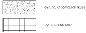
1. PROVIDE GYP. BD. AND RESILIENT CHANNELS CONTINUOUS AT BOTTOM OF FLOOR FRAMING TO MEET FIRE ASSEMBLY REQUIREMENTS. ALL SUSPENDED & FURRED CEILING TO BE BELOW COMPLETED FIRE RATED ASSEMBLY.
