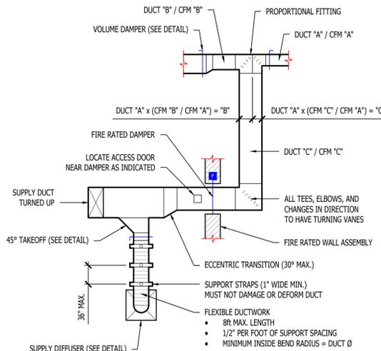
**TYPICAL DUCTWORK DETAIL**
