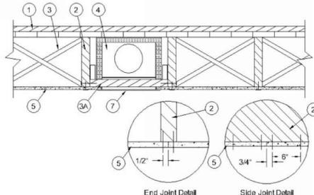
1. Flooring Systems — The flooring system shall consist of one of the following:
