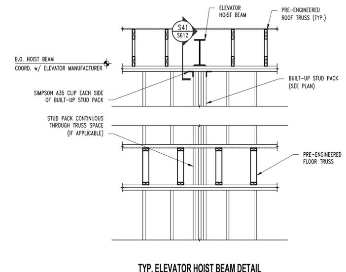
**TYP. ELEVATOR HOIST BEAM DETAIL**
