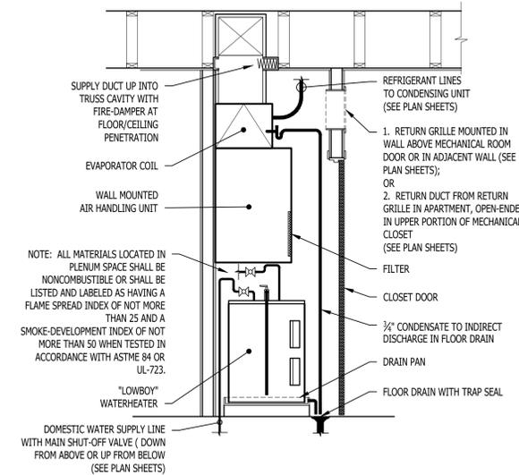
**STACKED WATER HEATER / AHU DETAIL**
