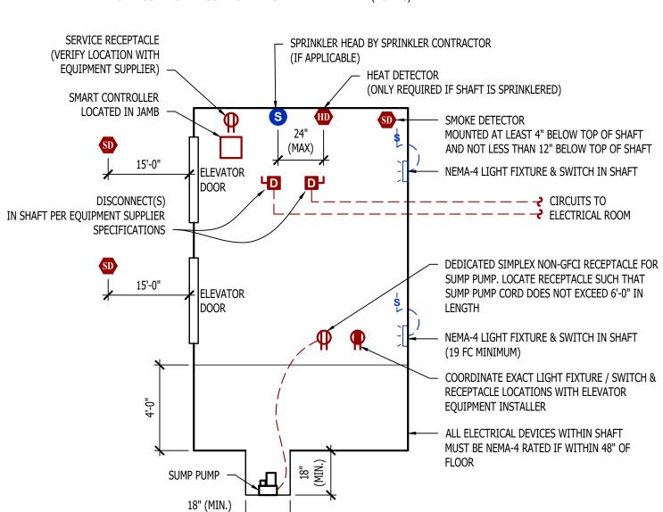
**MACHINE - ROOM - LESS ELEVATOR DETAIL**
