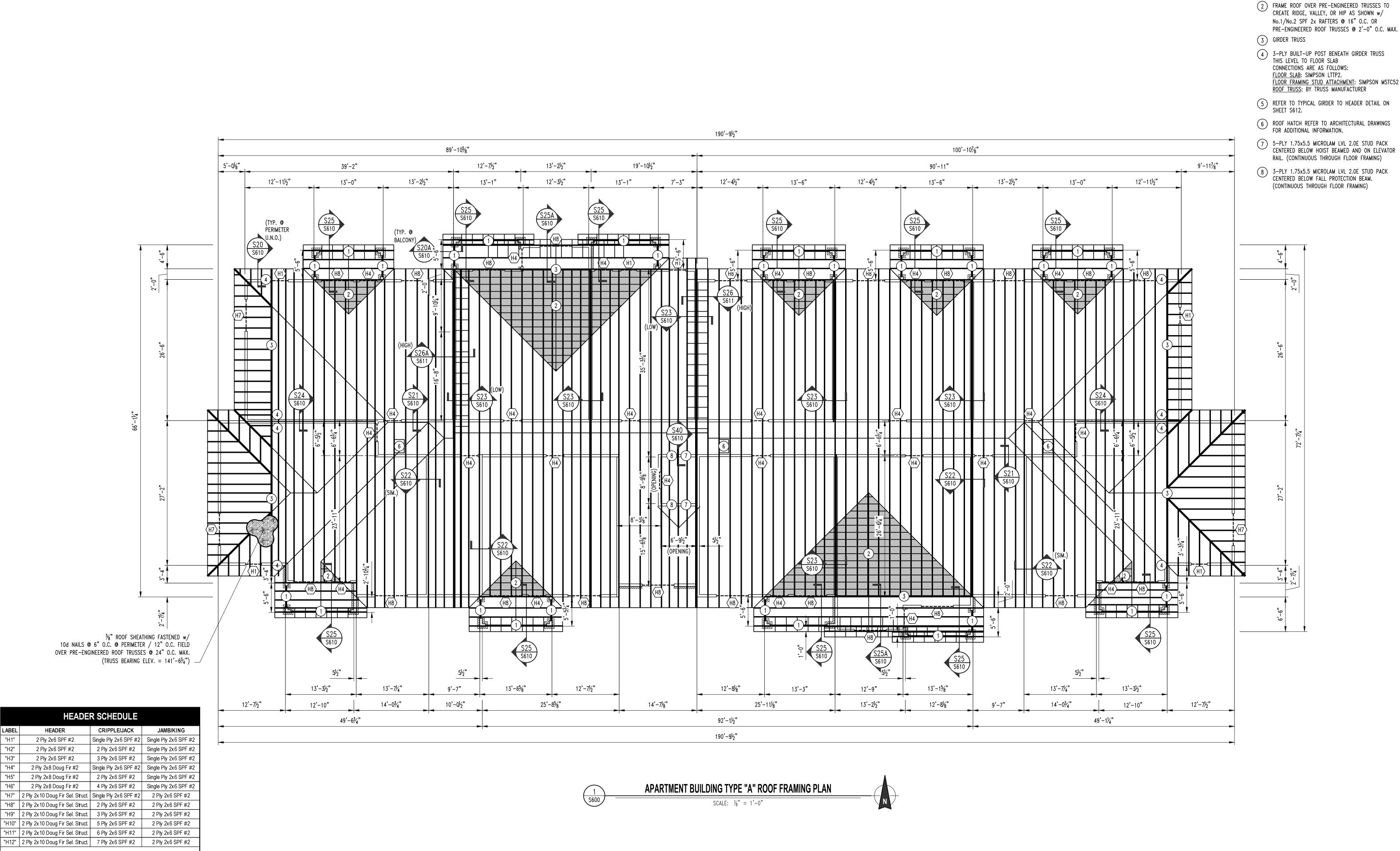
ALL DIMENSIONS ARE FROM FACE OF FOUNDATION WALL OR FRAMING;
