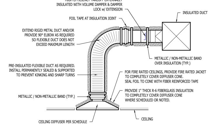
TYPICAL LAY-IN DIFFUSER DETAIL
