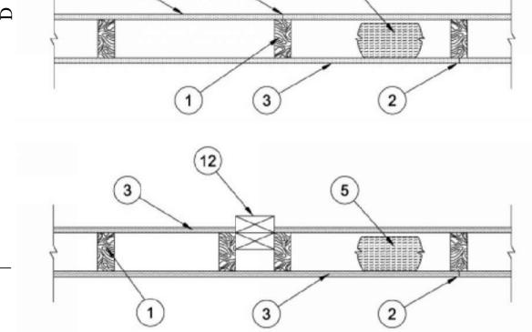
1. Wood Studs — Nom 2 by 4 in. spaced 16 in. OC max, effectively firestopped.
