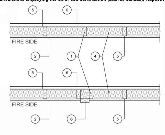
1. Wood Studs — Nom 2 by 4 in. spaced 16 in. OC with two 2 by 4 in. top and one 2 by 4 in. bottom plates. Studs laterallybraced by wood structural panel sheathing (Item 5). When Mineral and Fiber Boards\* (Item 5A) are considered as bracing for the studs, the load is restricted to 76% of allowable axial load. Walls effectively fire stopped at top and bottom of wall.
