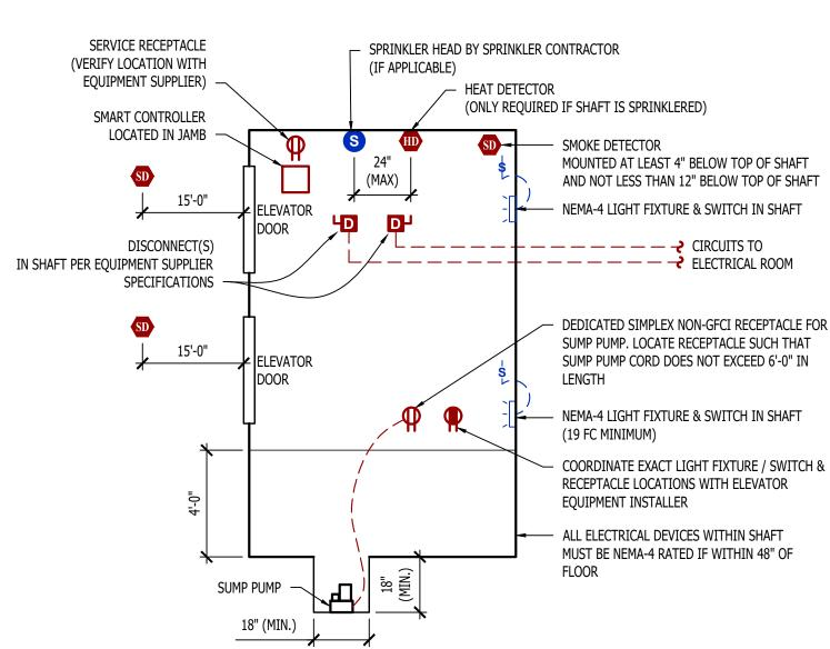
**MACHINE - ROOM - LESS ELEVATOR DETAIL**
