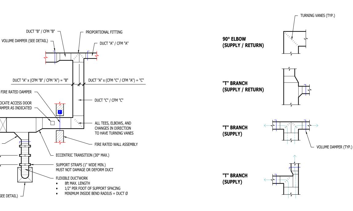
TYPICAL DUCTWORK DETAIL TYPICAL DUCTWORK FITTINGS DETAIL
