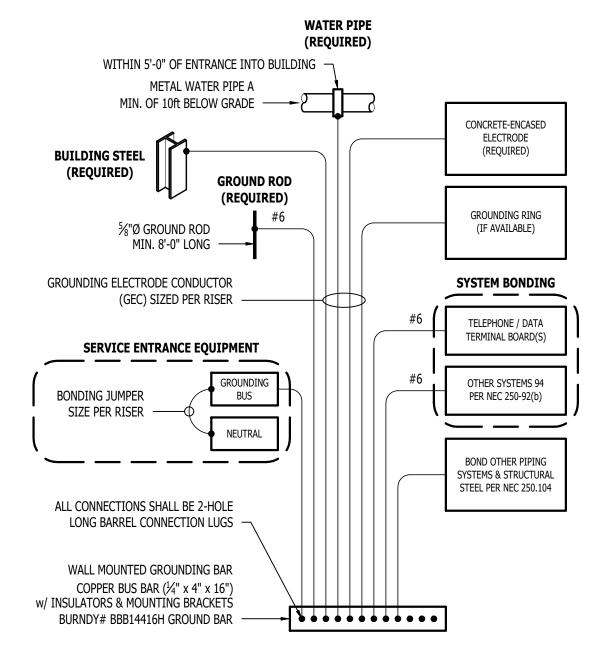
TYPICAL GROUNDING & BONDING DETAIL
