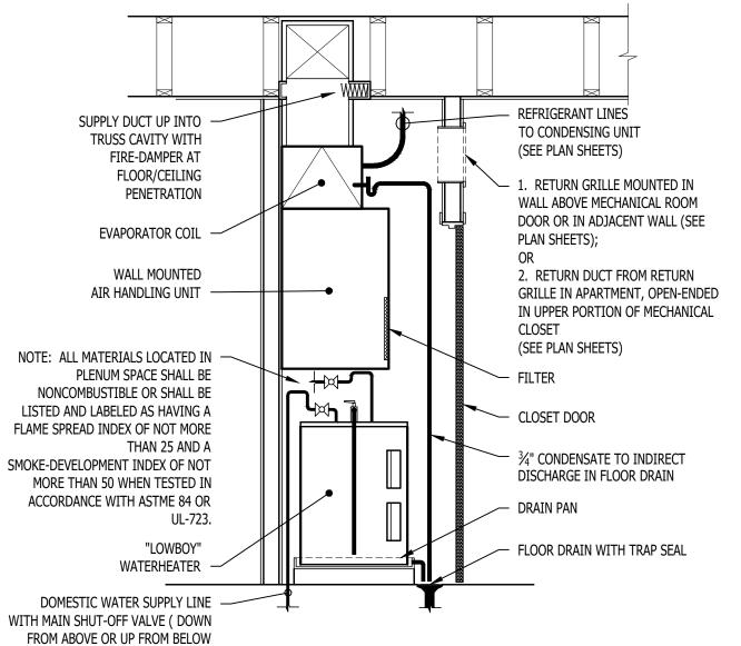
STACKED WATER HEATER / AHU DETAIL
