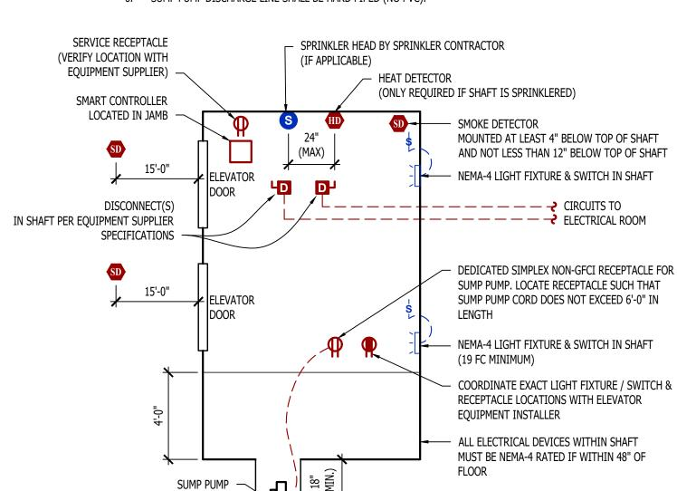
**MACHINE - ROOM - LESS ELEVATOR DETAIL**
