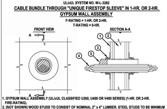
3-1/2" WIDE. 3. UNIQUE FIRESTOP PRODUCTS, DIVISION OF "IT'S UNIQUE" INC. SMOOTH SLEEVE, THREADED SLEEVE, OR SPLIT SLEEVE (2" AND 4" SIZES). 4. CABLE BUNDLE TO BE A COMBINATION OF ANY OF THE FOLLOWING:
