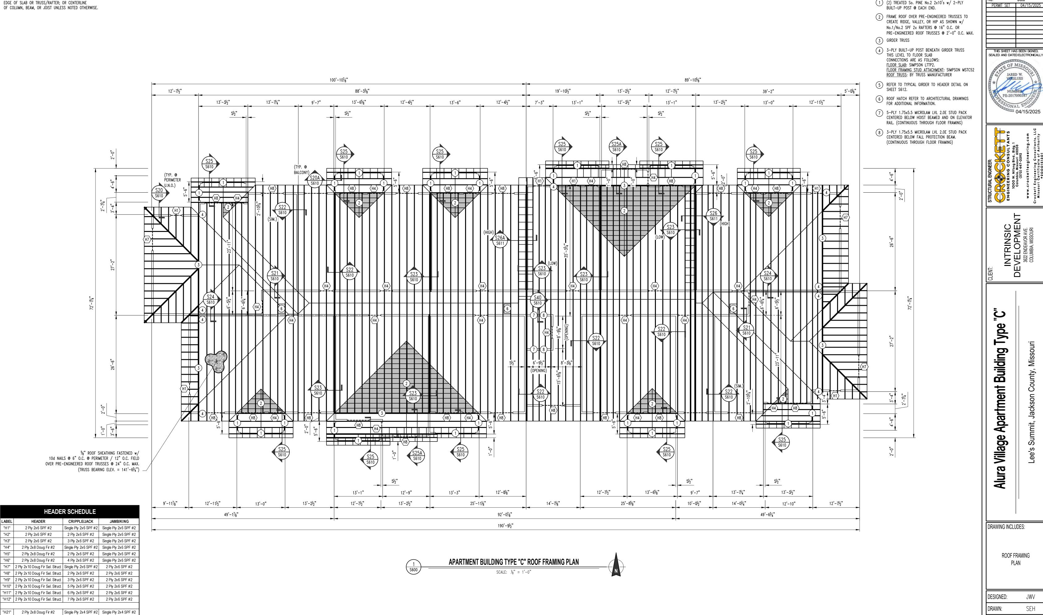
ALL DIMENSIONS ARE FROM FACE OF FOUNDATION WALL OR FRAMING;
