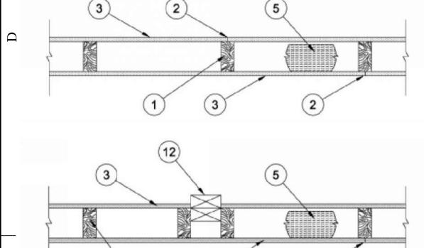
1. Wood Studs — Nom 2 by 4 in. spaced 16 in. OC max, effectively firestopped.
