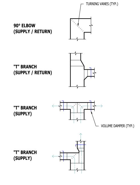
TYPICAL DUCTWORK FITTINGS DETAIL
