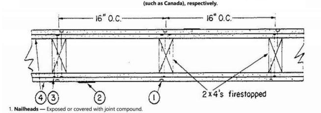
2. Joints — Exposed joints covered with joint compound and paper tape. Joint compound and paper tape may be omitted when square edge boards are used. As an alternate, nom 3/32 in. thick gypsum veneer plaster may be applied to the entire surface of Classified veneer baseboard with the joints reinforced with paper tape.
