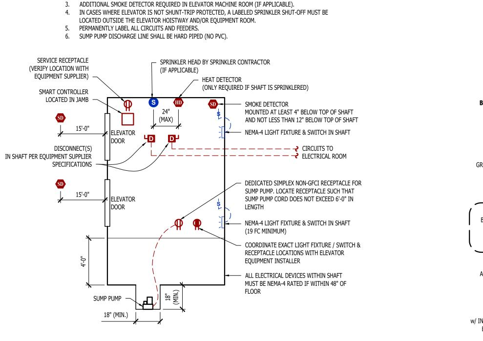
MACHINE - ROOM - LESS ELEVATOR DETAIL
