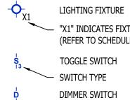
── "X1" INDICATES FIXTURE TYPE (REFER TO SCHEDULE) TOGGLE SWITCH - SWITCH TYPE
