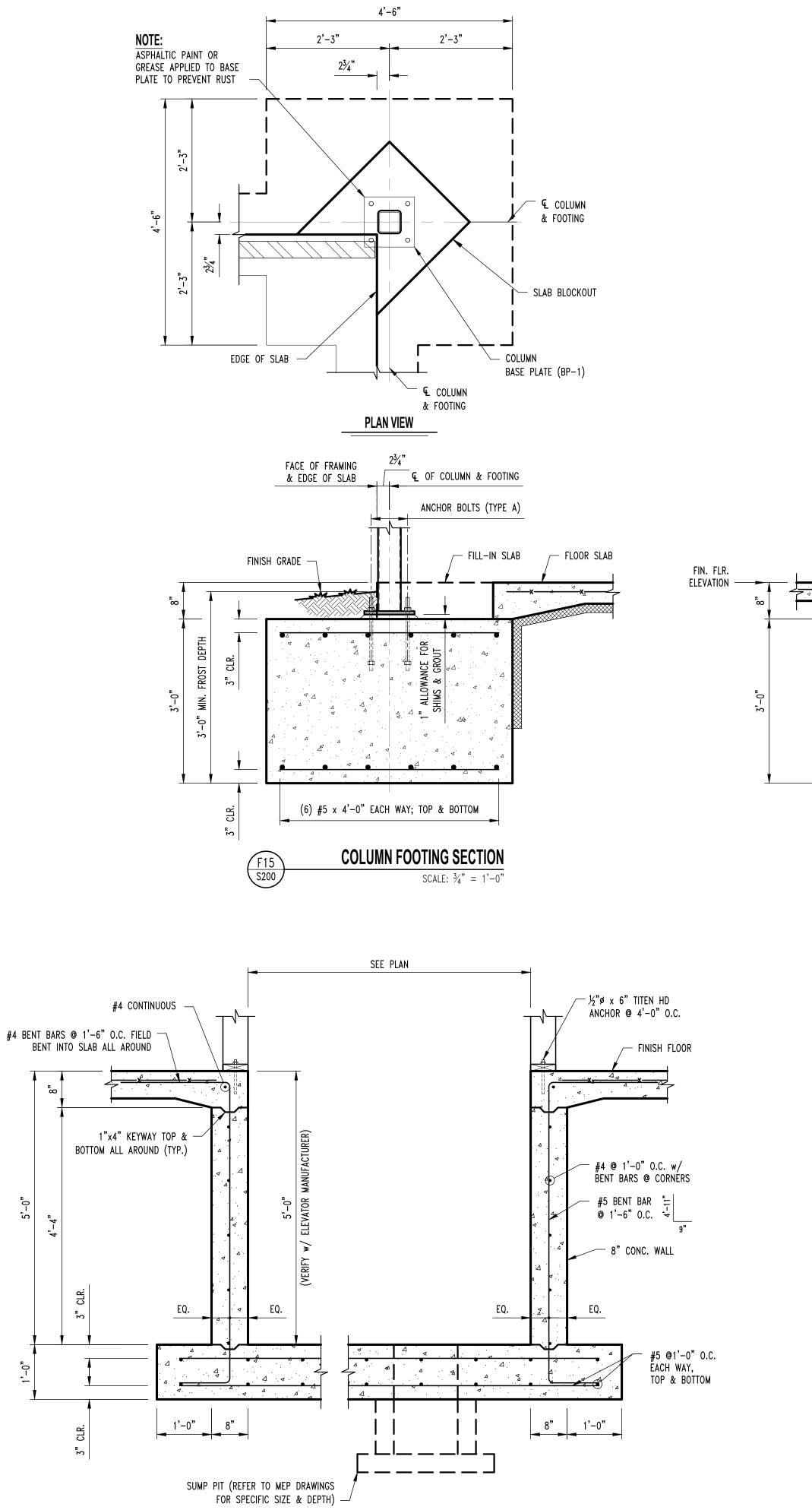
**ELEVATOR PIT SECTION** SCALE:  $\frac{3}{4}$ " = 1'-0"
