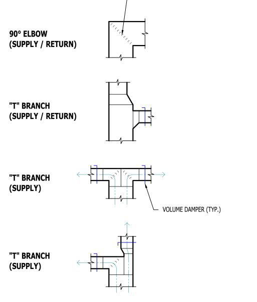
TYPICAL DUCTWORK FITTINGS DETAIL
