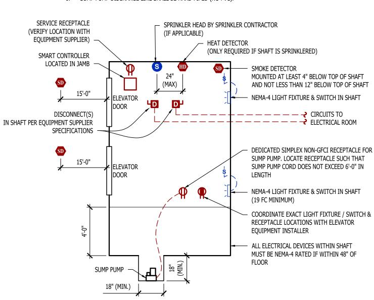
**MACHINE - ROOM - LESS ELEVATOR DETAIL**
