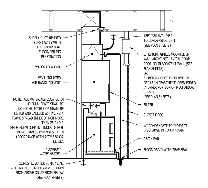
STACKED WATER HEATER / AHU DETAIL
