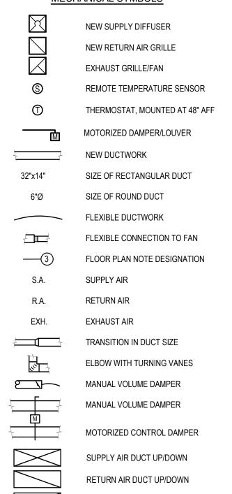
EXHAUST AIR DUCT UP/DOWN
