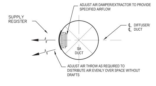
SUPPLY REGISTER DETAIL SCALE: NONE
