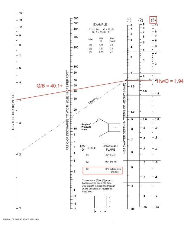
Figure 5603-1: Headwater Depth for Box Culverts with Inlet Control
