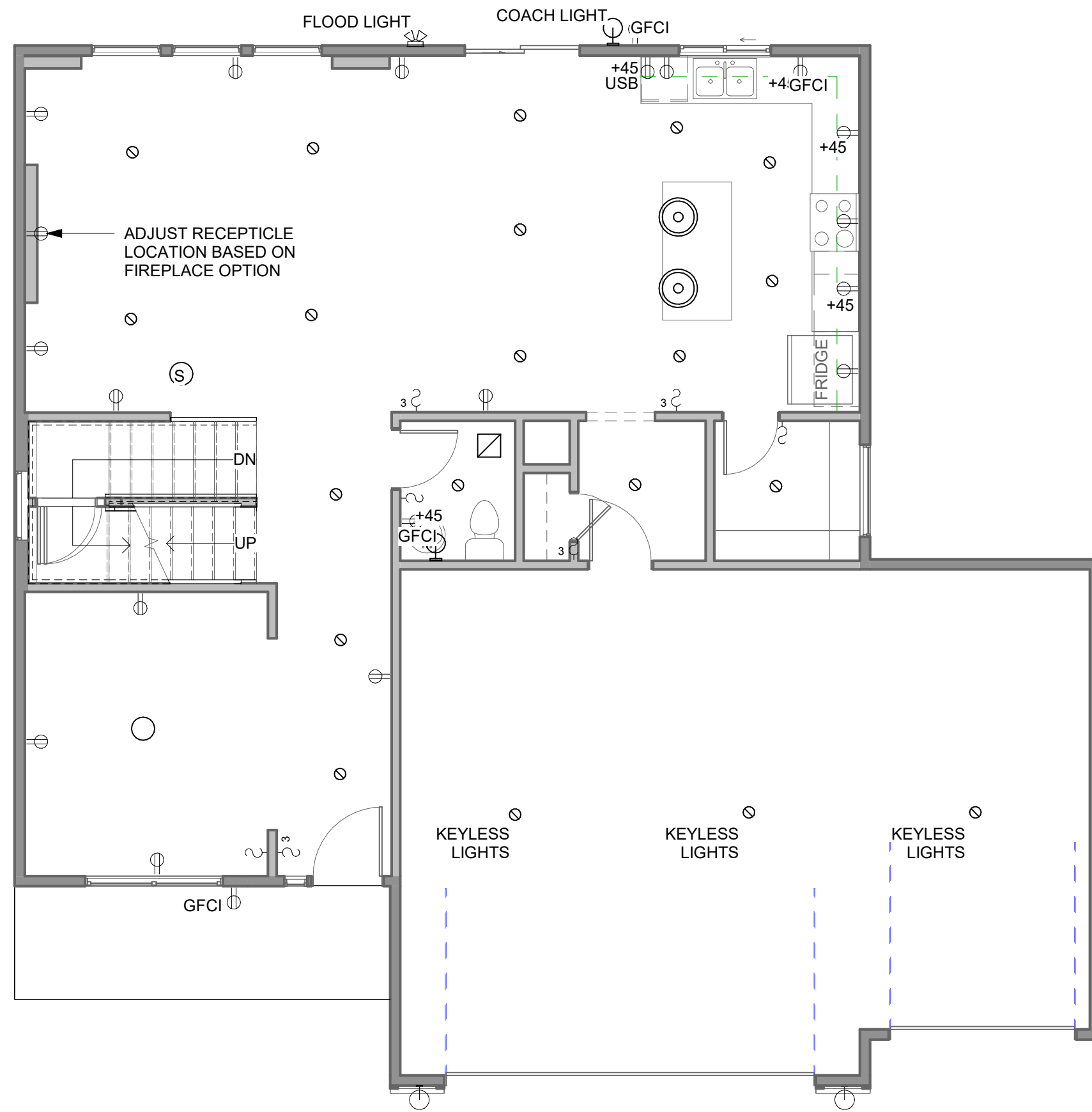
2 PLAN VIEW - MAIN LEVEL LIGHTING/OUTLET 3RD BAY 3/16" = 1'-0"
