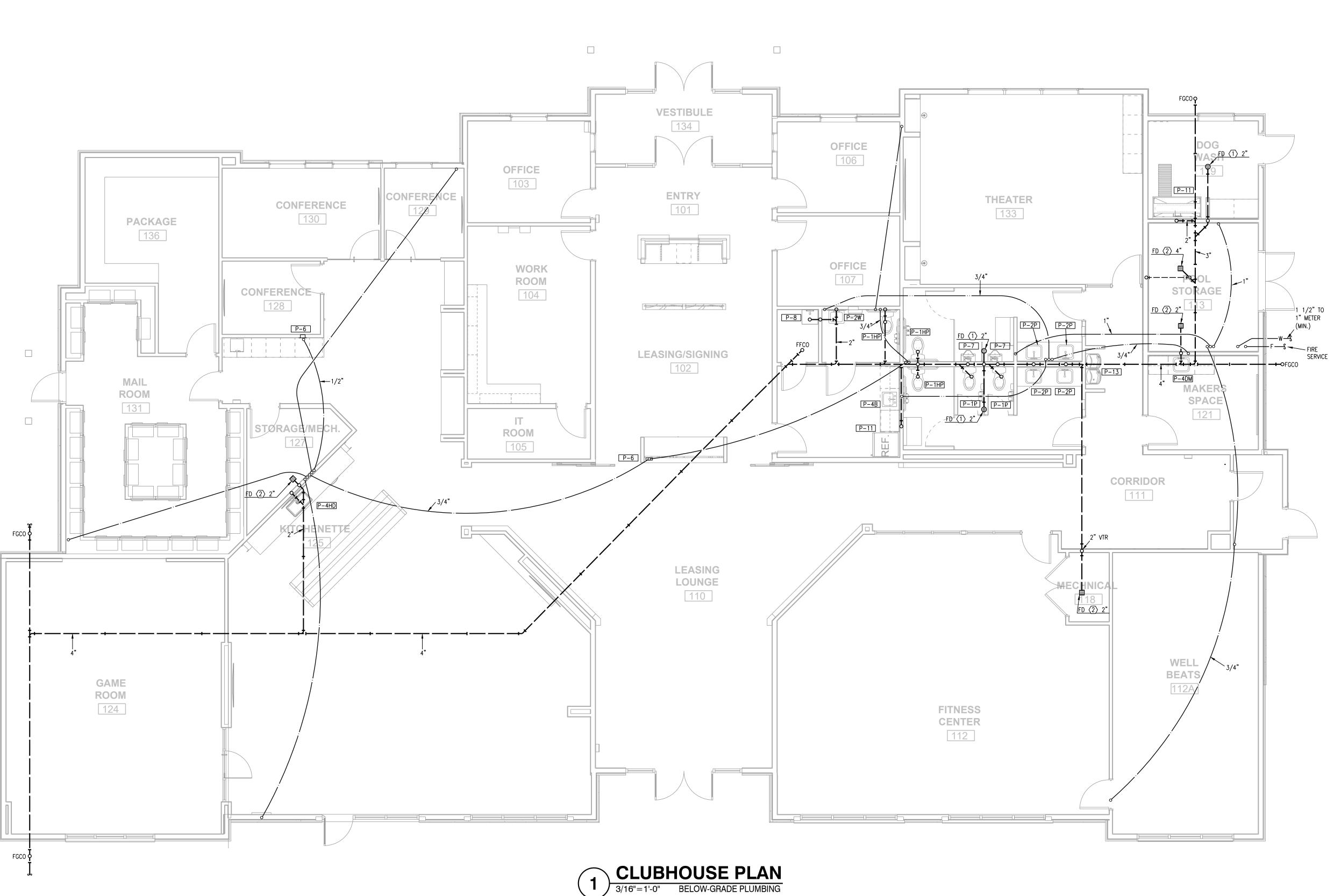
ALL DRAIN, WASTE AND VENT PIPING IS 2" UNLESS NOTE OTHERWISE.
