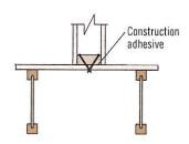
Nail interior partitions to the joists when possible. If the wall can be nailed only to the floor panel, run a bead of adhesive\* under the wall and either cross nail, nail through and clinch tight, or screw tightly into the wall from below.
