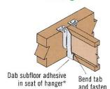
Seat the joist tight to the bottom of the hanger. When using hangers with tabs, bend the flange tabs over and nail to the TII® joist bottom flange. Placing a dab of sublfoor adhesive\* in the seat of the hanger prior to installing the joist can reduce squeaks.
