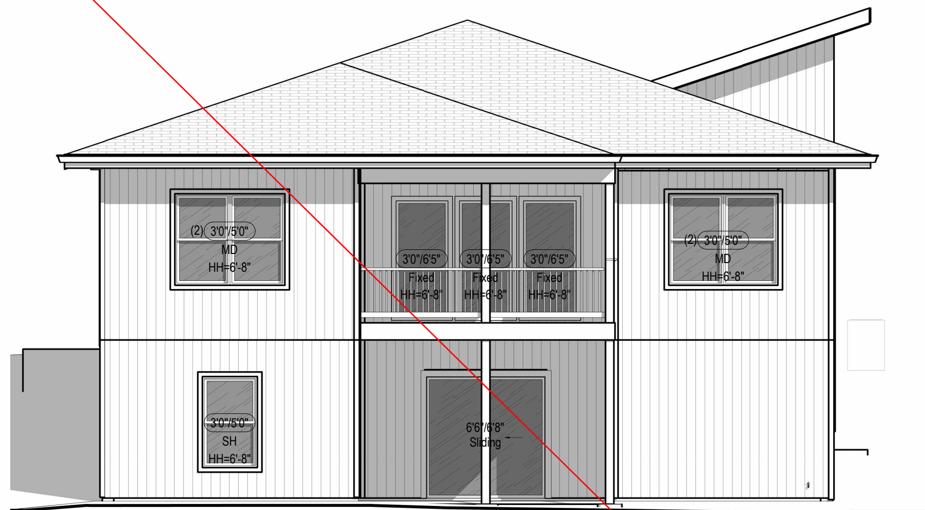
6 Back Elevation - Deck for Walkout Basement - shed - Full covered Deck 3/16" = 1'-0"
