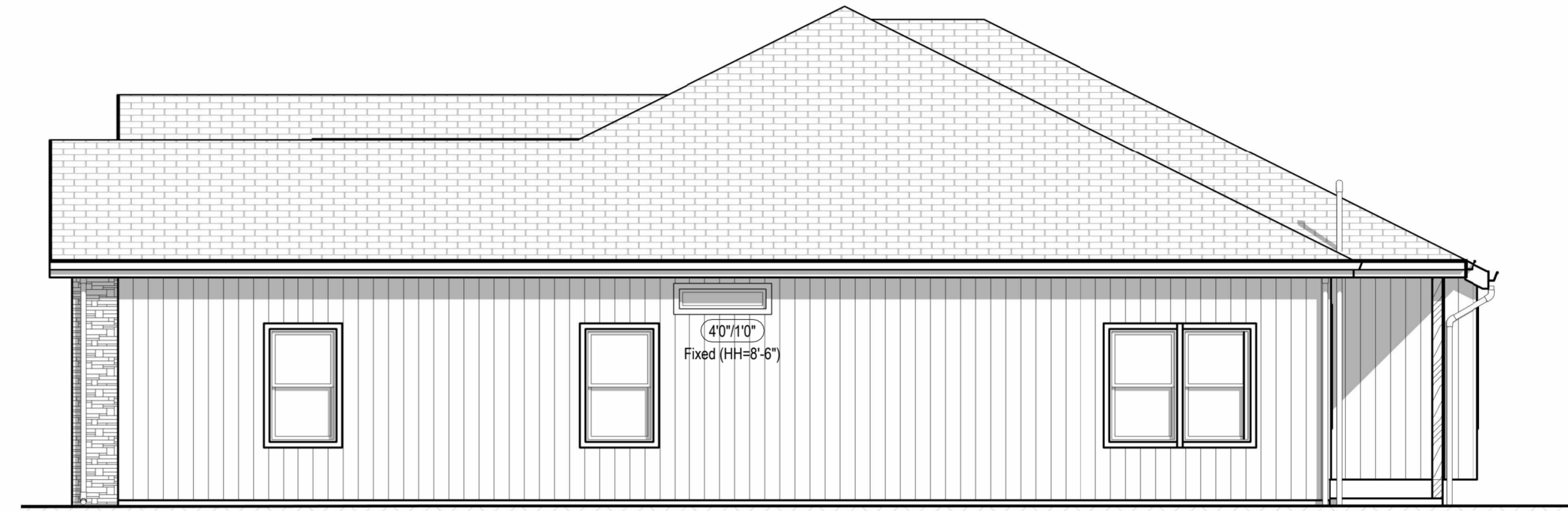
4 Right Elevation (Full Basement) - Transitional 3/16" = 1'-0"
