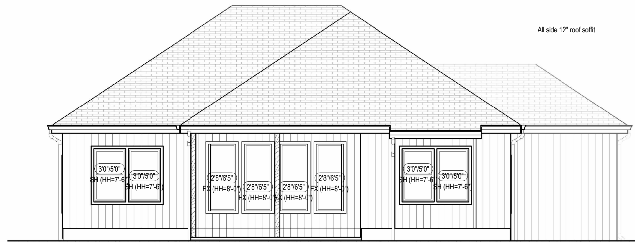
7 Rear Elevation (Full Basement) - Transitional 3/16" = 1'-0"
