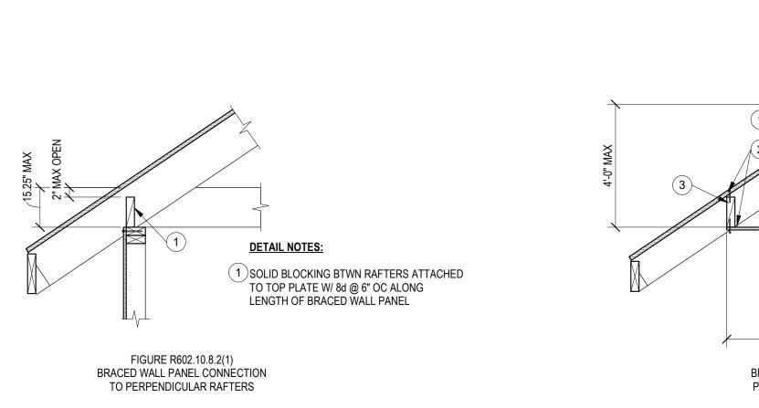
6'-0" MAX FIGURE R602.10.8.2(2) BRACED WALL PANEL CONNECTION OPTION TO PERPENDICULAR RAFTERS OR ROOF TRUSSES
