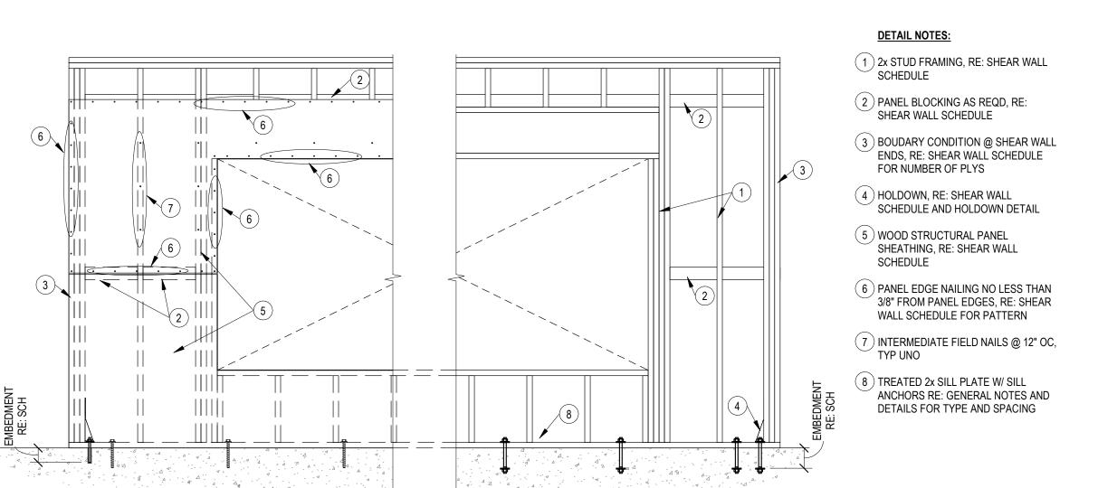
PERFORATED SHEAR WALL - ELEVATION
