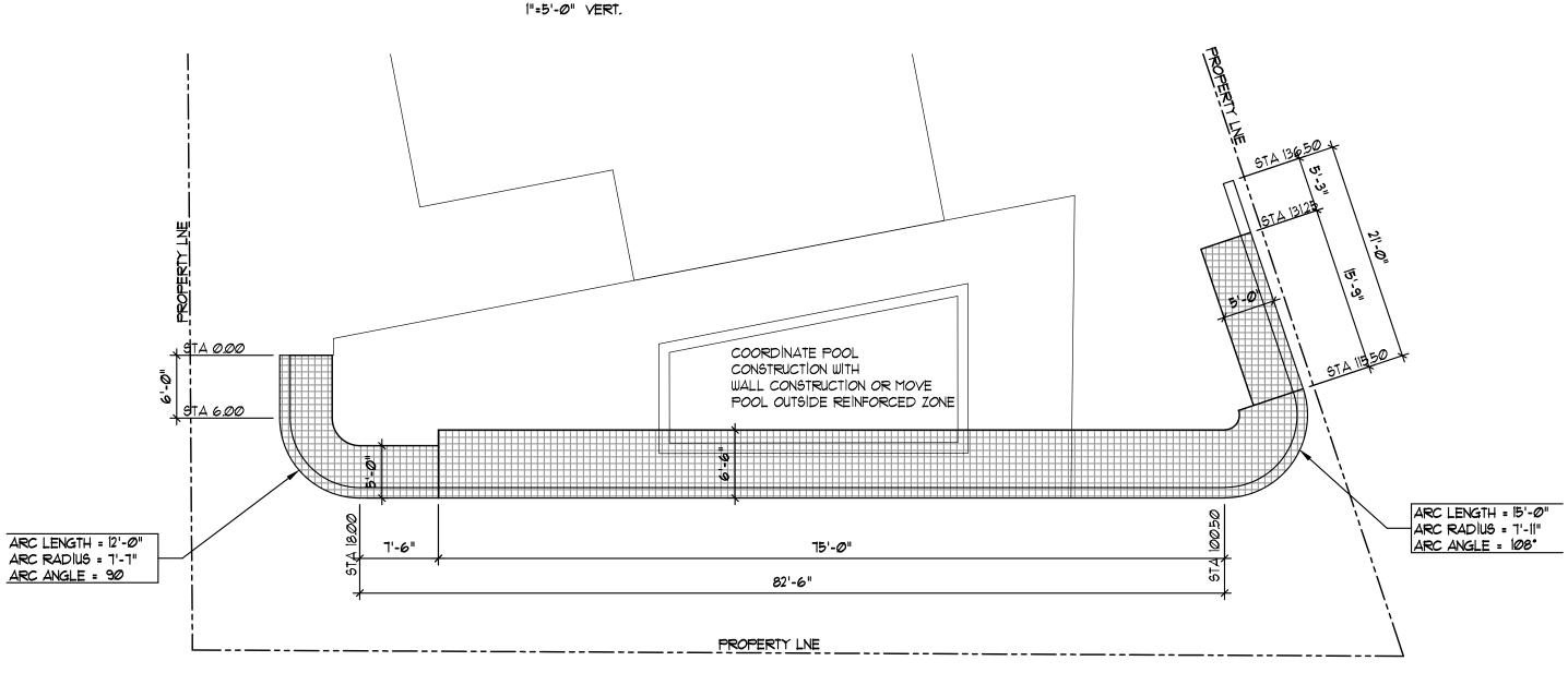
REINFORCED SOIL RETAINING WALL PLAN (NORTH)
