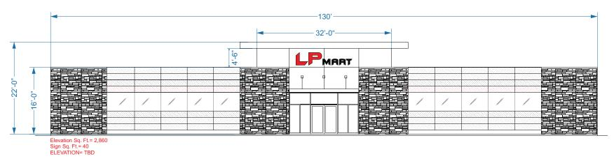
Fabricate & Install: Internally Illuminated 3" deep, flush mounted. 3/16" white acrylic faces.
