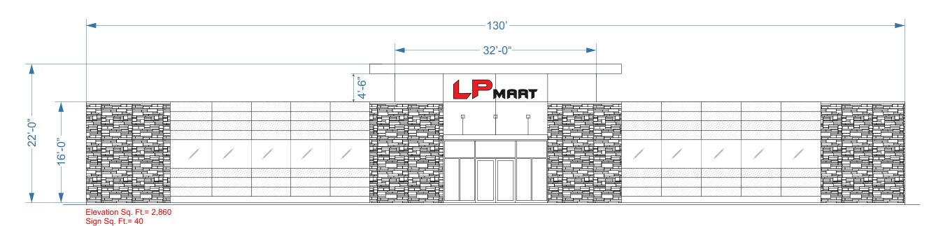
Fabricate & Install: Internally Illuminated 3" deep, flush mounted. 3/16" white acrylic faces.
