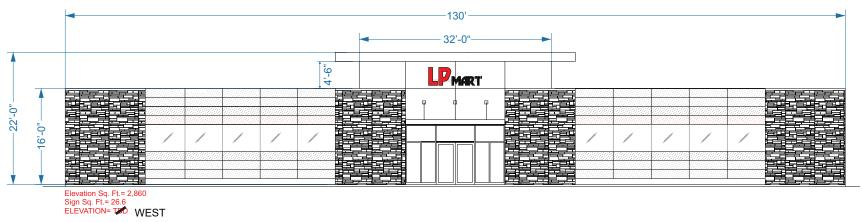
Fabricate & Install: Internally Illuminated 3" deep Channel Letters mounted to raceway.
