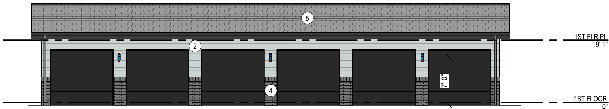
4 GARAGE 2 - FRONT ELEVATION 1/8" = 1'-0"
