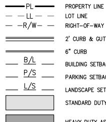
2' CURB & GUTTER \_\_\_\_\_ <u>B/L</u> \_\_\_\_\_ BUILDING SETBACK LINE \_\_\_\_\_ <u>P/S</u> \_\_\_\_\_ parking setback line \_\_\_\_ <u>L/S</u> \_\_\_\_ LANDSCAPE SETBACK LINE STANDARD DUTY ASPHALT PAVEMENT HEAVY DUTY ASPHALT PAVEMENT PROPOSED BUILDING CONCRETE PAVEMENT
