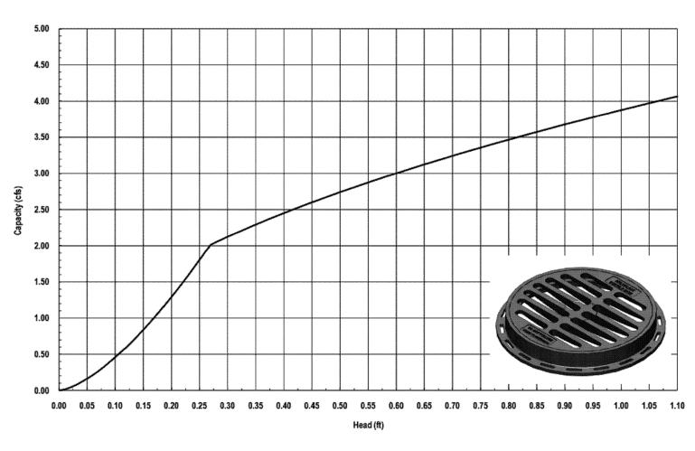
ALL SECONDARY STORM INLETS WILL CAPTURE 0.01-0.03 ACRES OF RUNOFF RESULTING IN < 0.5 CFS DURING THE 100-YEAR STORM. THIS WILL RESULT IN LESS THAN 0.1 FT OF HEAD OVER THE INLET PER THE CAPACITY CALCULATION ABOVE.
